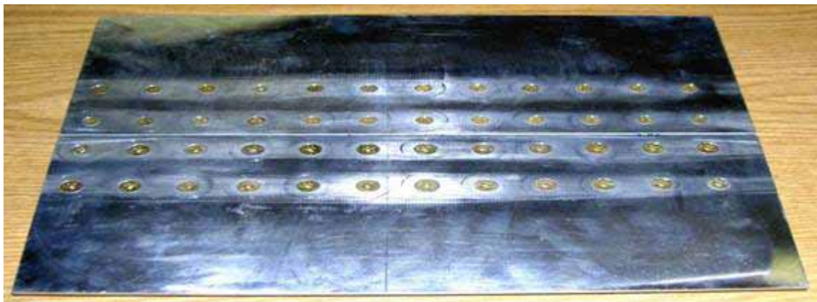
Figure 21. KC-135 360 Wing Splice sample. There are three layers on the left, and two on the right. The horizontal gap has a crack in the second layer. Fasteners are ferrous, and several cracks have been cut into the second layer. The lower two rows of fasteners are larger than the upper two rows.
