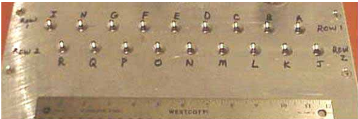
Figure 13. Photo of upper layer of the modular samples. The two staggered rows of 0.375" holes are countersunk to accommodate flush fasteners. The dimensions of the sample are 15" long, by 8" wide, by 0.350" thick. All of the interchangeable lower layers are 15" long, by 4" wide, by 0.395" thick.
