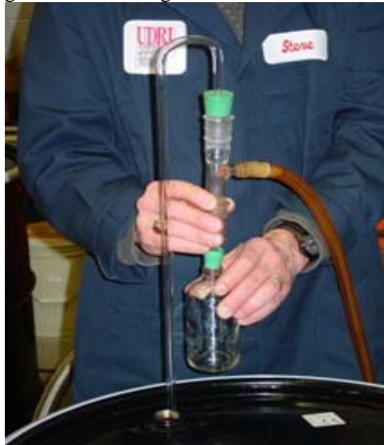
Figure 3: Fluid sampling from drum using the vacuum connector method
