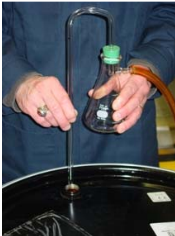
Figure 2: Fluid sampling from drum using the vacuum flask method
