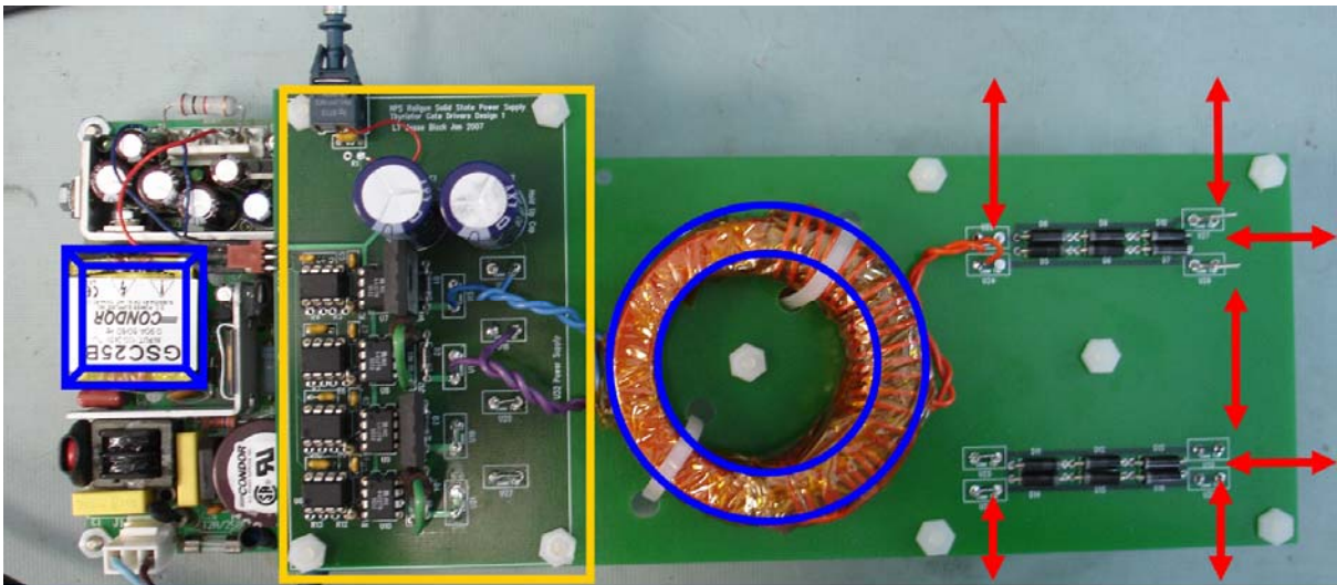
Figure 25. EMP Suppression and Creepage and Clearance.
