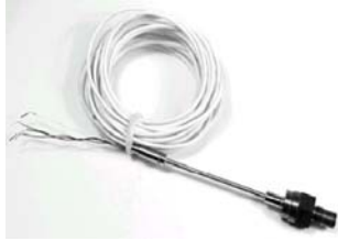
Packaged 6H-SiC pressure sensors were tested at temperatures higher than 500°C on a turbine engine
