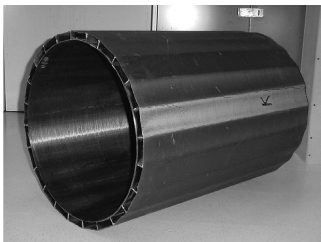
Fig. 2 Early chamber core structure used for noise reduction experiments.
