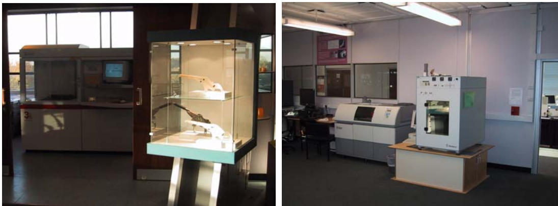
Figure B.14. Loughborough's Rapid Manufacturing Lab machines: ( left ) Stereolithography SLA 7000; ( right ) ThermoJet Concept Modeler.
