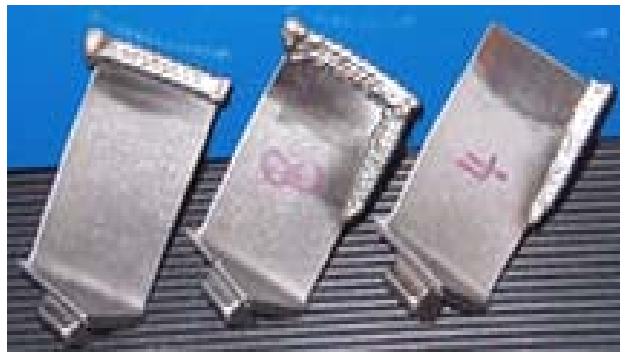
Figure B.23. Turbine blades with laser cladding build-up.
