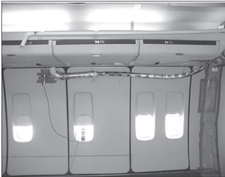
Figure 4. Graphic illustrating introduction of VHP stream into AERF through nominal 4-in diameter duct. a) (above) global view facing cabin sidewall, b) (lower left) view upwards towards overhead luggage carrier, c) (lower right) view towards rear of cabin showing injection angle.
