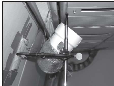
Figure 4. Graphic illustrating introduction of VHP stream into AERF through nominal 4-in diameter duct. a) (above) global view facing cabin sidewall, b) (lower left) view upwards towards overhead luggage carrier, c) (lower right) view towards rear of cabin showing injection angle.
