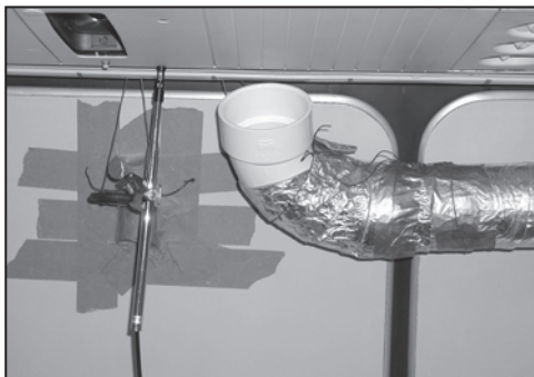
Figure 4. Graphic illustrating introduction of VHP stream into AERF through nominal 4-in diameter duct. a) (above) global view facing cabin sidewall, b) (lower left) view upwards towards overhead luggage carrier, c) (lower right) view towards rear of cabin showing injection angle.
