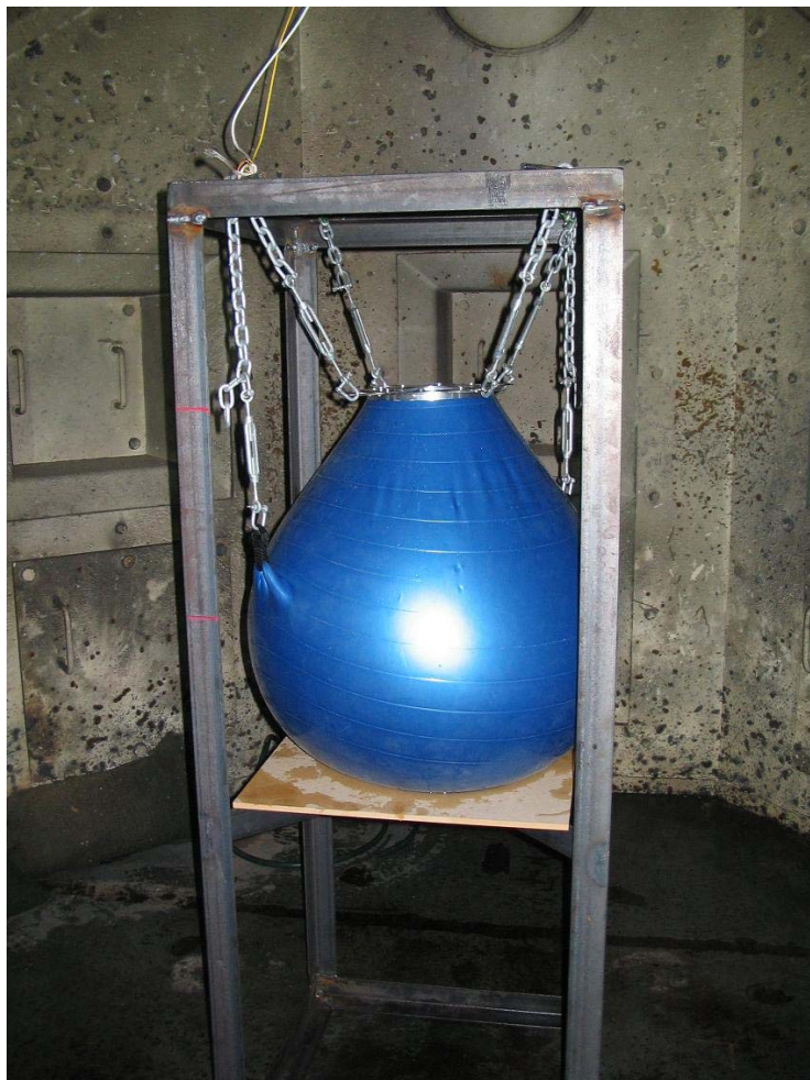
Figure 7. Charge set-up for tests with an explosive charge submerged in bulk liquid
