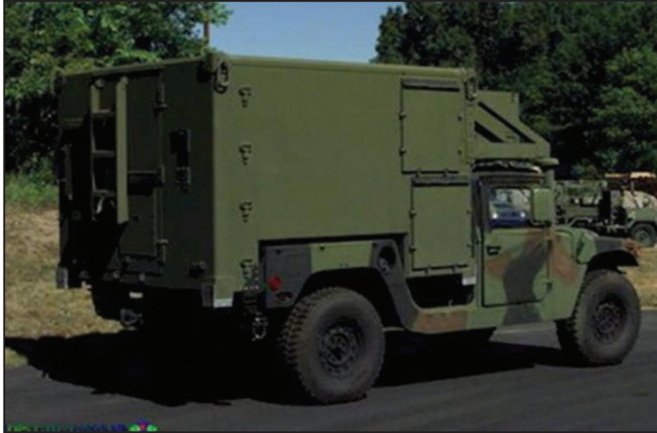
Figure D-18. Single Shelter Switch AN TTC 56
