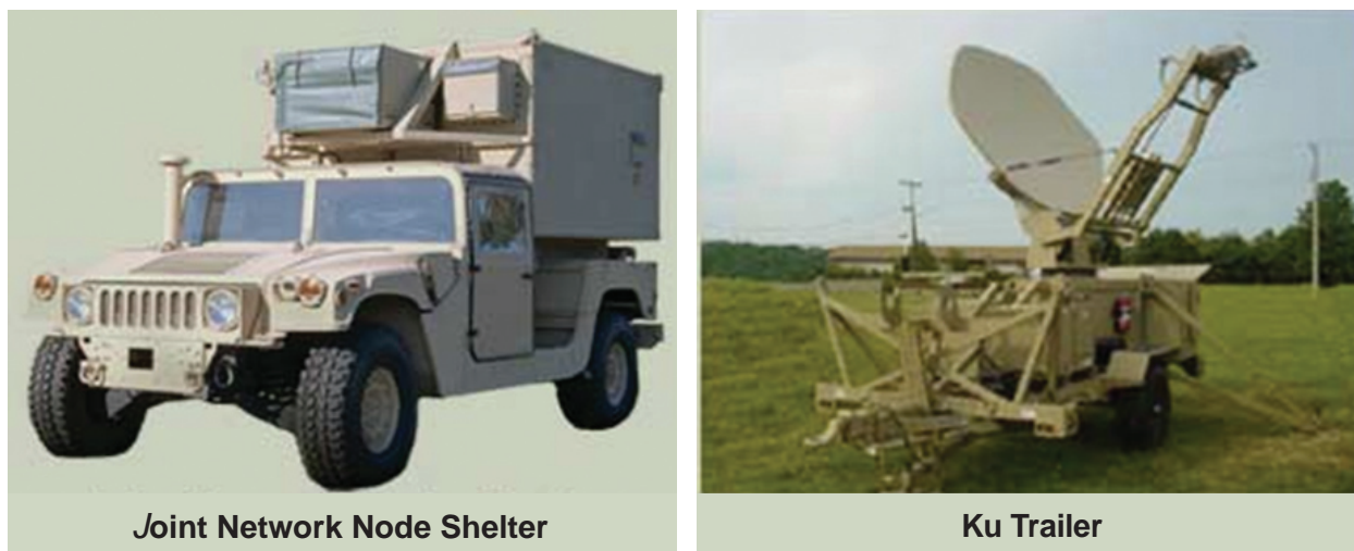
Figure 26. A Joint Network Node Communications Shelter and Satellite Terminal Trailer.
