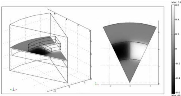
Figure 4. FEMLAB finite element model results showing the z-directed B field 100  $\mu\text{m}$  above the stator surface for the case of  $p=8$ .
