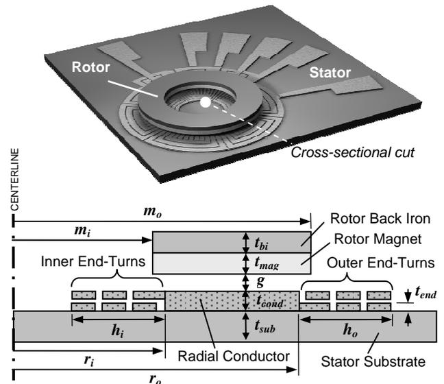
Figure 1. Axial-flux permanent-magnet machine perspective and cross-sectional schematics.
