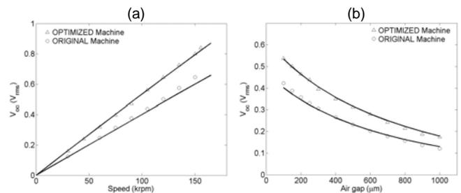
Figure 7. Open-circuit voltages (a) vs rotational speed for 100  $\mu\text{m}$  air gap and (b) vs. air gap at 100,000 rpm for original and optimized machines. Data points represent measurements; lines represent analytical model.
