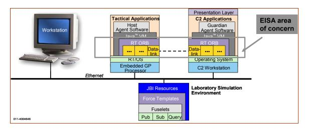
Figure 5 Conceptual SIRES Testbed Architecture
