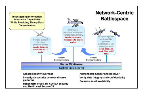
Figure 2 Time-critical Target Scenario in a Network-centric Battlespace
