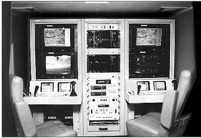
Figure 7. Control station for the Predator UAS.
