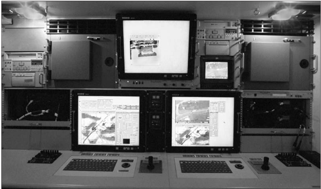
Figure 1. Control station for the Shadow UAS.
