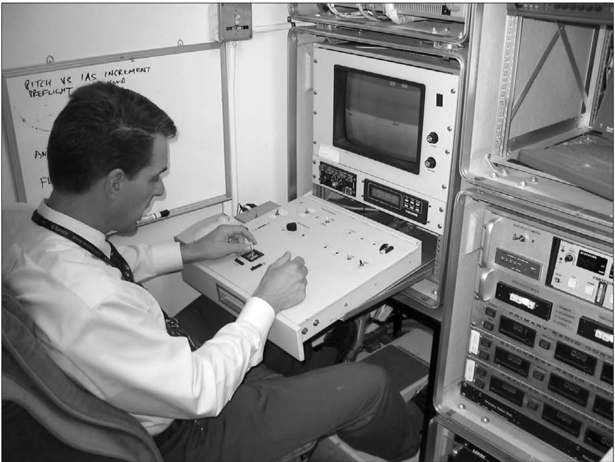
Figure 8. Control interface for the Perseus UAS.
