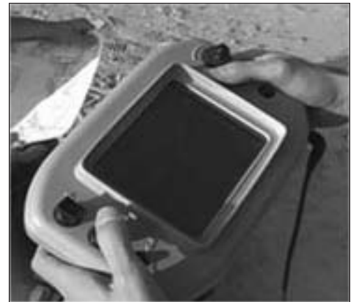
Figure 6. Control box for Raven and Puma UAS.
