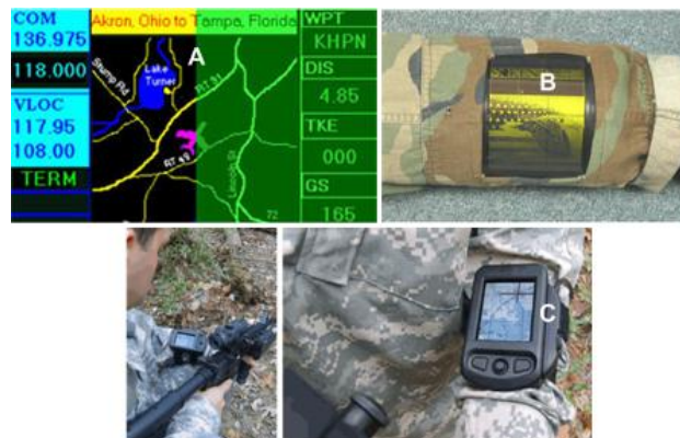
Figure 20 – A) Kent Infrared Display; B) Kent Flexible Display; and C) Trident Enclosure w/ Controls
