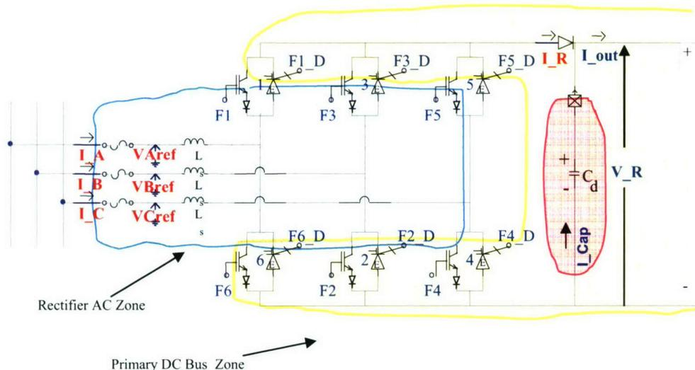
Figure 2.4 : Protection zones around Rectifier PEBB
