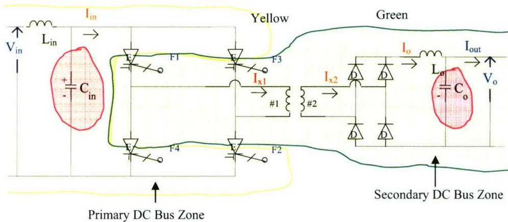
Figure 2.12 : Buck Converter Associated Protection Zones
