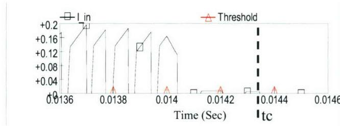
Figure 2.15 : Buck Converter Source side fault
