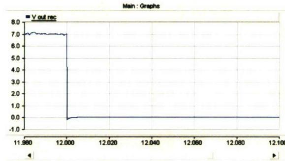
(a) Rectifier output voltage (voltage in kV, time in sec).
