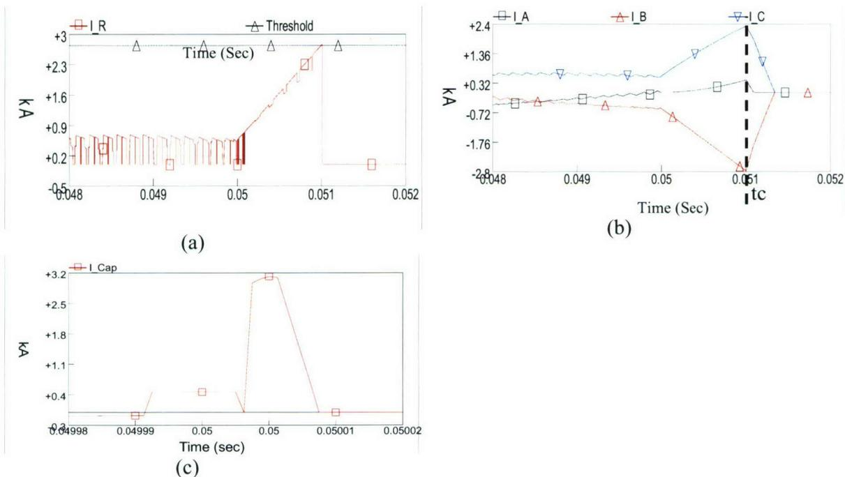
Figure 2.6 : Simulation results of Rectifier DC Bus fault
