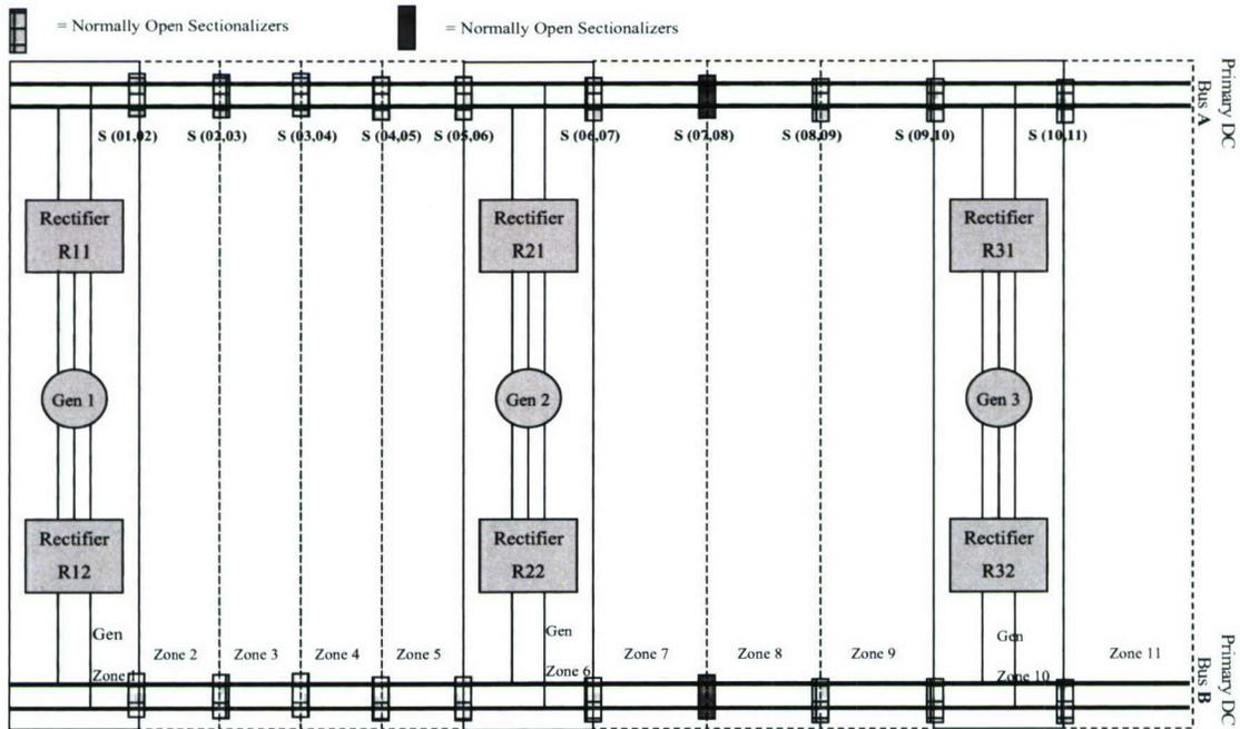
Figure 4.1: Shipboard Electrical System with Three Generator Configuration
