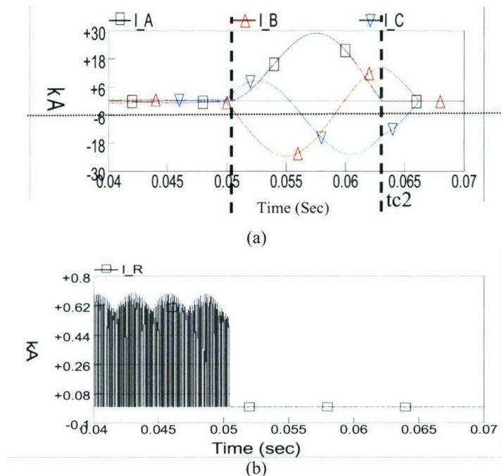
Figure 2.10 : Simulation results of 3-phase fault
