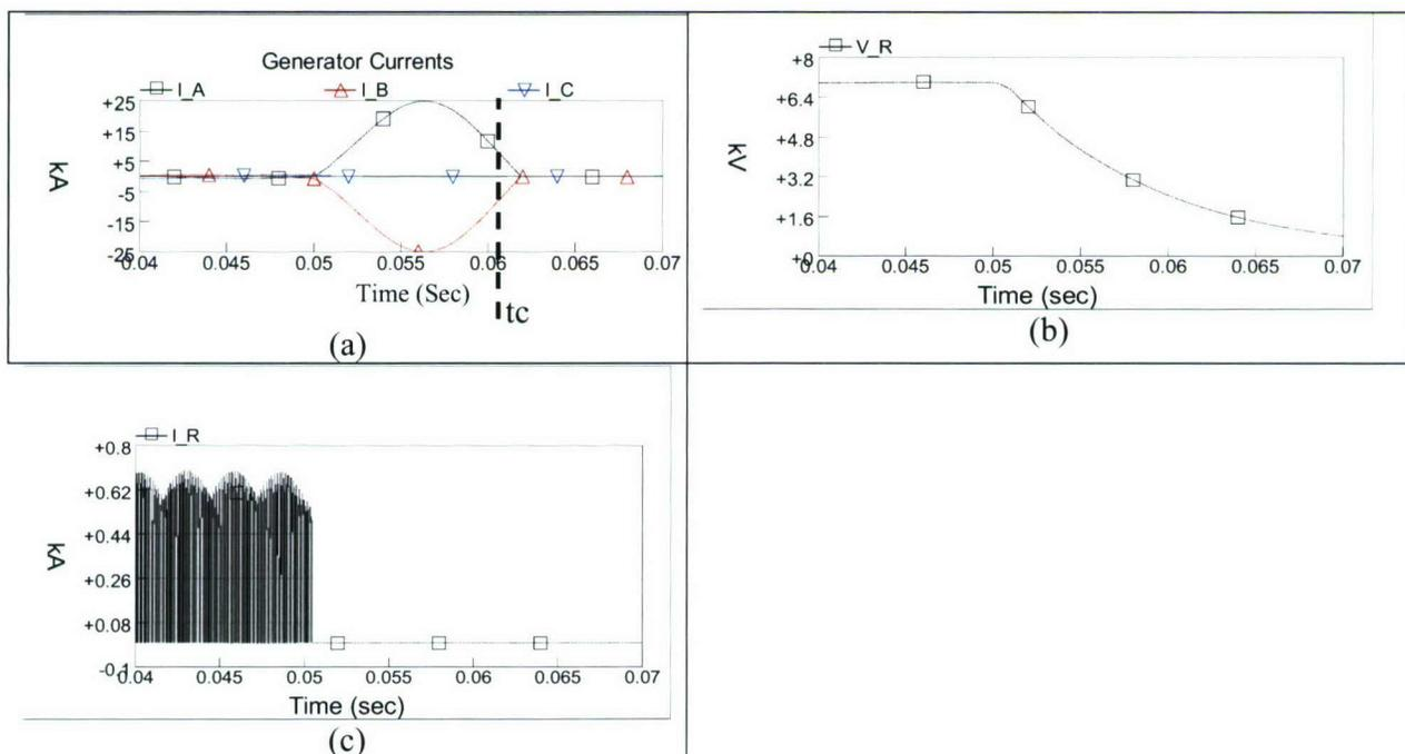
Figure 2.9 : Simulation results of L-L fault before Inductor
