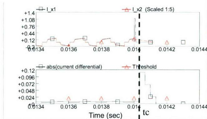
Figure A.17 : Transformer Primary side Fault Detection
