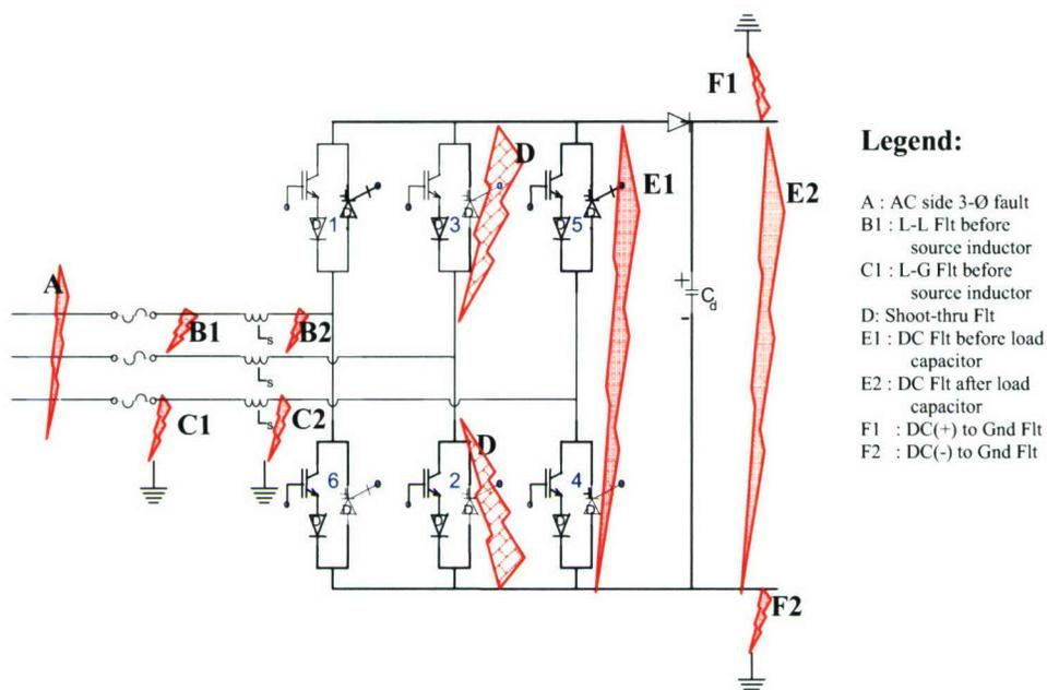
Figure 2.5 : Faults close to Rectifier PEBB
