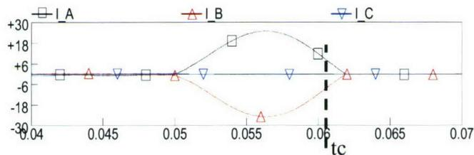
Figure 2.3 : Fuse Operation to clear a L-L fault.
