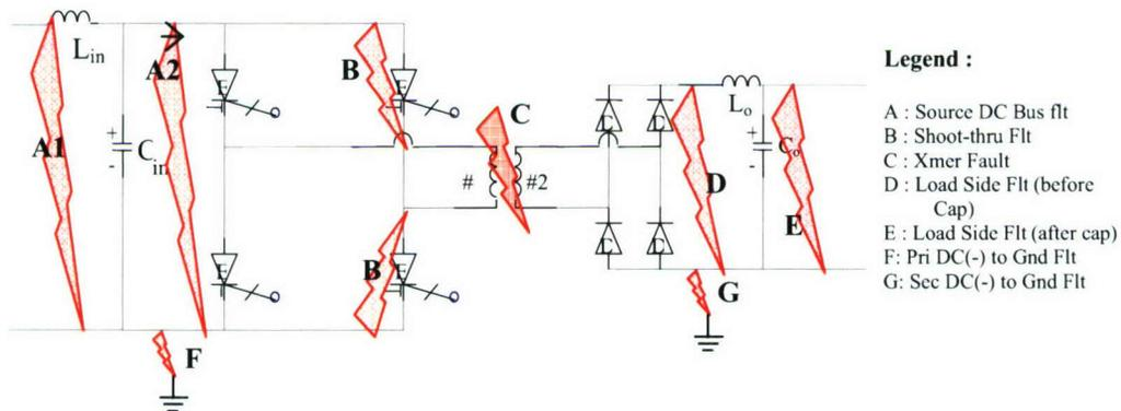
Figure 2.13 : Faults close to Buck Converter PEBB
