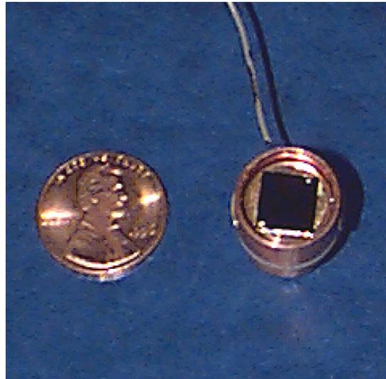
Fig 6: A photograph of a multiple quantum well modulator.
