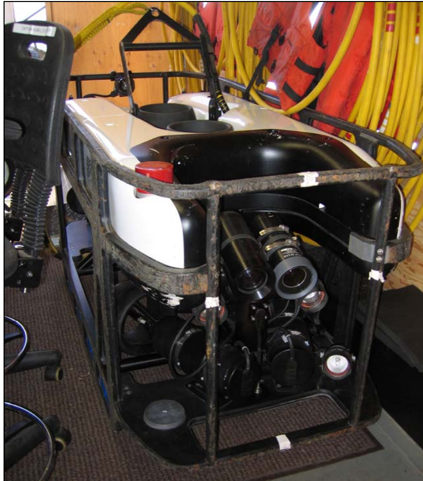
Figure 6. Front view of Chelan PUD's custom-made ROV used for turbine inspections.
