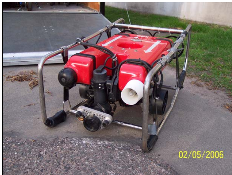
Figure 2. Deep Ocean Engineering Phantom 500XTL-380 ROV showing a camera, lasers, light, and compass mounted to the front of the vehicle.
