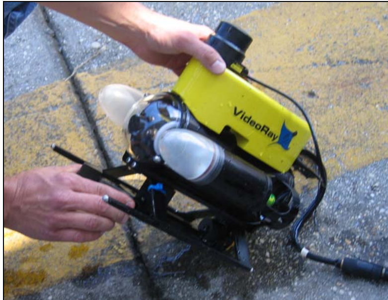
Figure 4. VideoRay Pro III used by the Mobile District. The operator's lower hand is holding a small gripper, and his upper hand is touching the scanning sonar head. This 8-lb ROV is easily deployed by one person.
