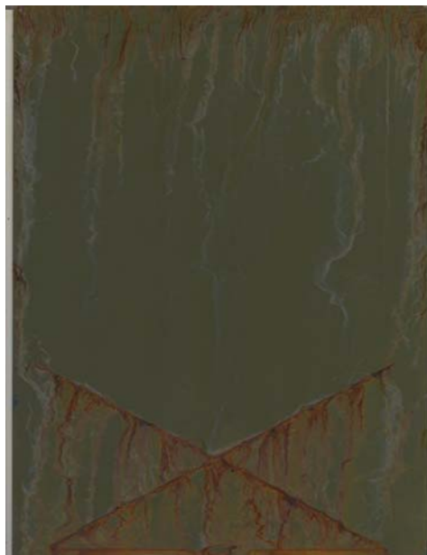
Figure 13. ASTM B117 (salt-fog results) CRS panels after 264-hr exposure.
