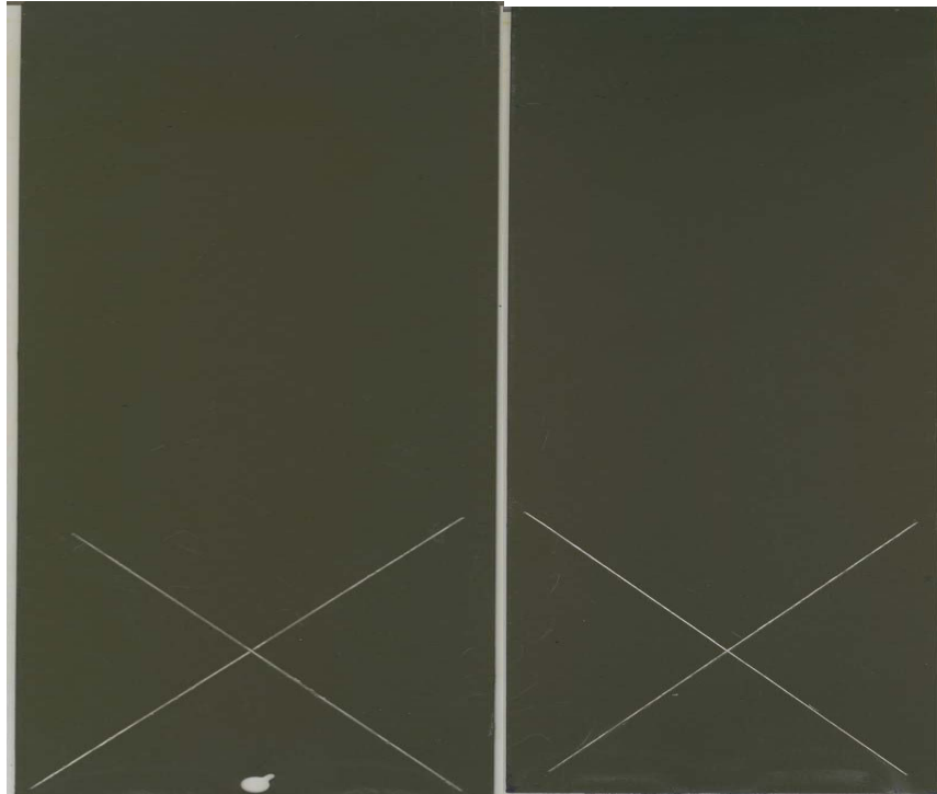
Figure 14. GM 9540 P (cyclic corrosion results) aluminum test panels after 10 cycles of exposure.
