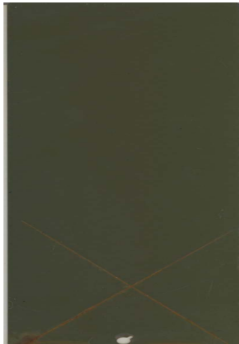
Figure 15. GM 9540 P (cyclic corrosion results) CRS test panel after 10 cycles of exposure.
