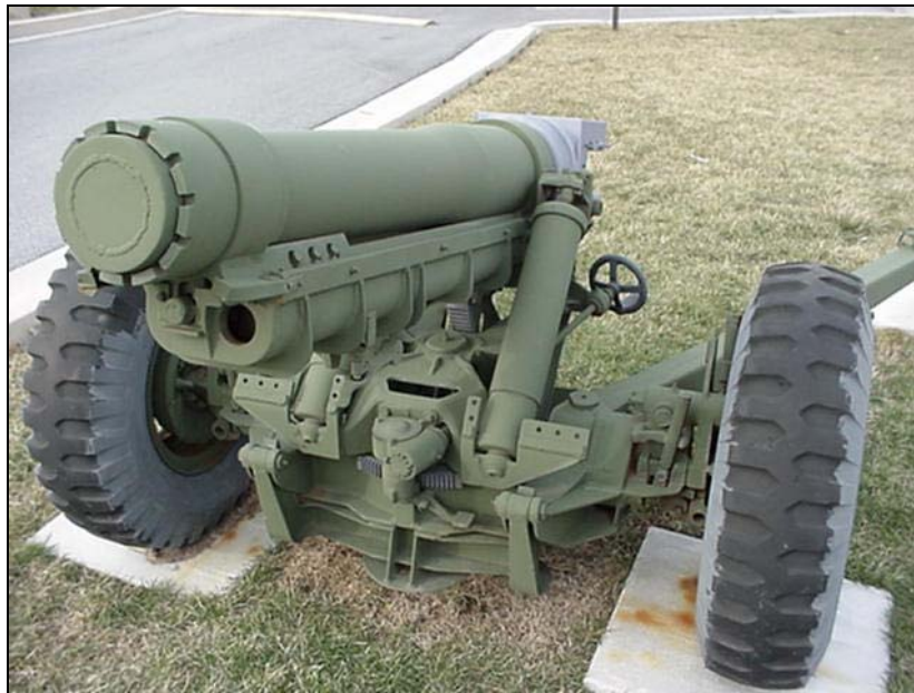
Figure 11. Water-reducible wash primer system; painted 8 December 2004.
