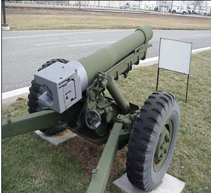
Figure 10. Water-reducible wash primer system; units were painted 8 December 2004.
