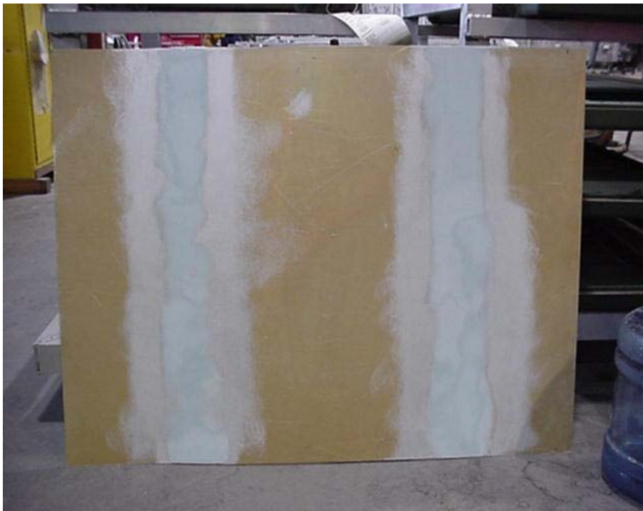
Figure 33. After body filler is feathered out (just before coating application).
