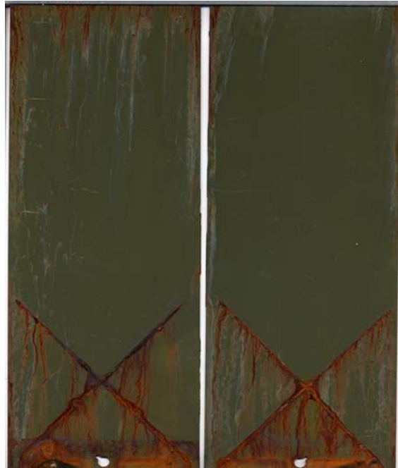
Figure 16. ASTM B117 after 1008-hr exposure. Steel panel without wash primer and with Sherwin Williams' KemAqua.
