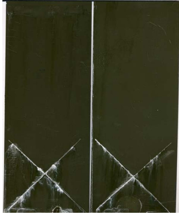
Figure 20. AL-2024-T3 GM 9540P at 1008 cycles.
