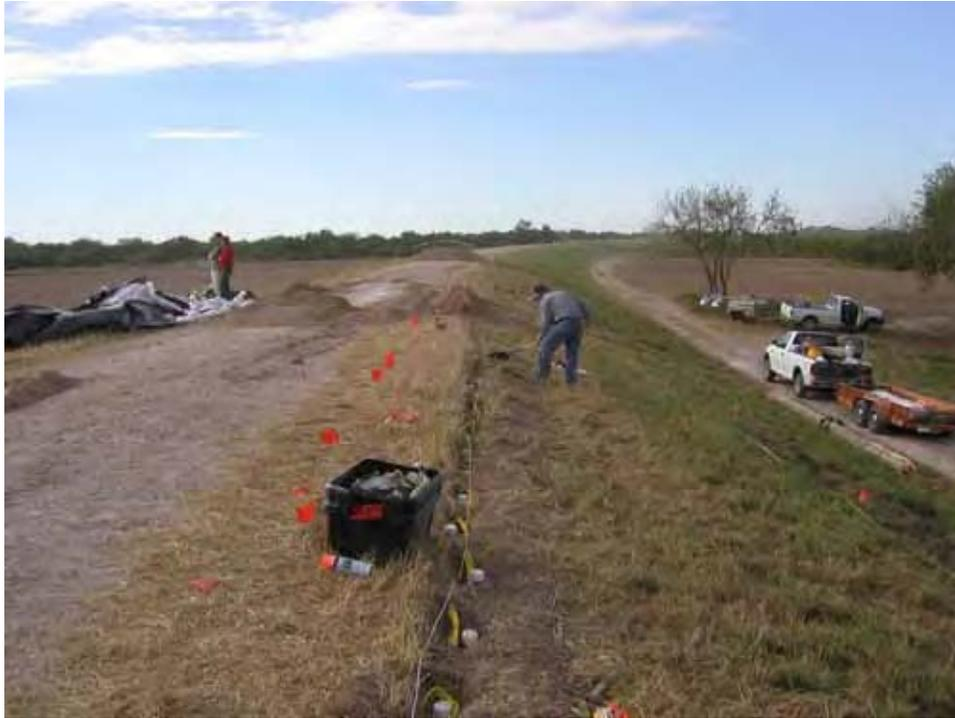
Figure 26. View of SP line (line A) looking upstream (west). Electrodes spacing is 2.5 ft, total length of line is 50 ft
