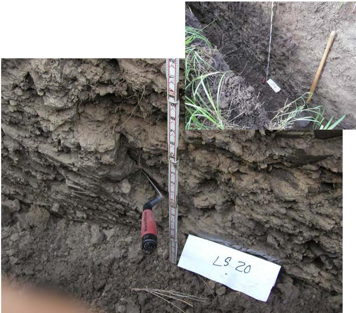
Station LS 20, photograph from 5. to 6 ft, crack near base of trench, note the blocky texture, soil is generally brittle and dry
