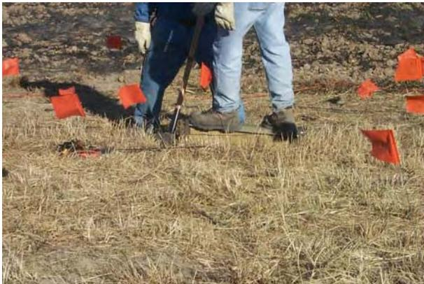
Figure 20. Shear-wave data acquisition, site 1.
