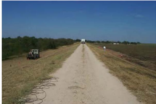
Figure 2. Field site 1 with vibrator on south side of levee, crew working on north side, and semi parked on levee.
