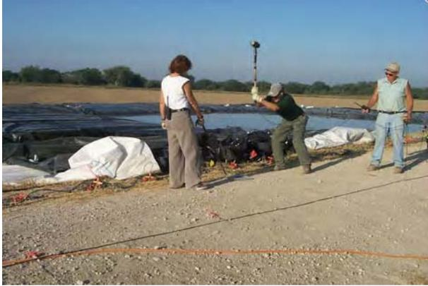
Figure 33. Compressional-wave survey during full pool.
