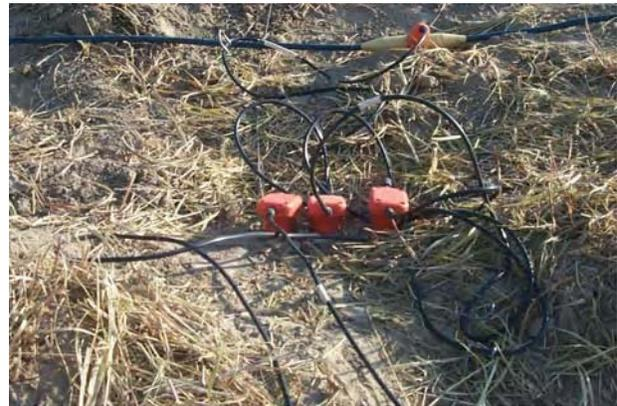
Figure 21. Compressional-wave phones used for through-levee, site 1.
