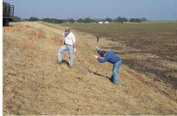
Figure 19. Compressional-wave data acquisition, site 1.
