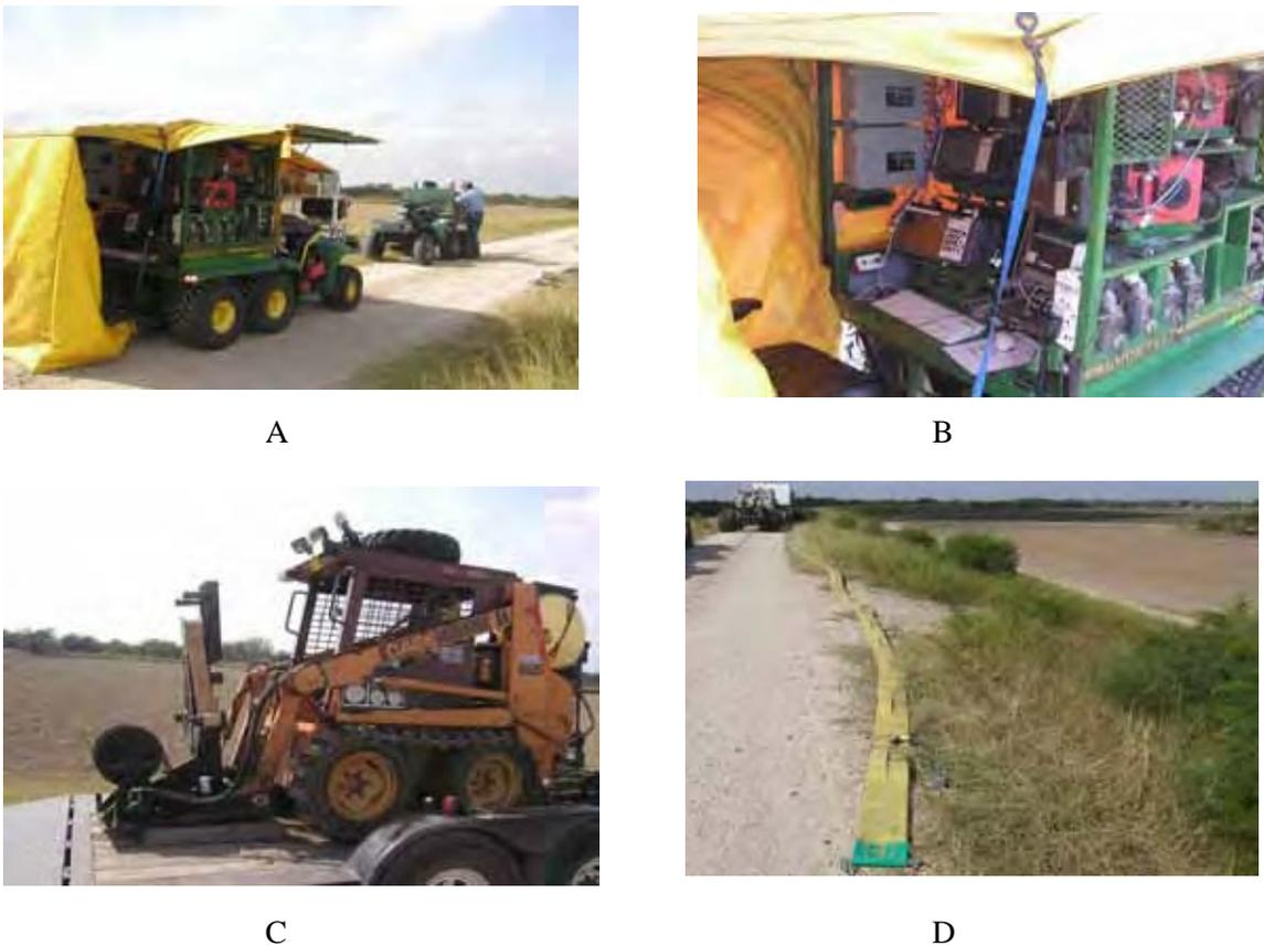
Figure 18. Seismic equipment used during investigations of IBWC levees: (A) seismic recording cart, (B) close-up view of seismographs in recording cart, and (C) seismic source for producing surface waves, (D) towed land streamer or geophones in fire-hose for rapid seismic surveying capabilities and fixed geophones (in blue, foreground) were evaluated
