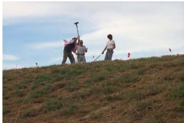
Figure 10. Compressional-wave survey along levee crest road.
