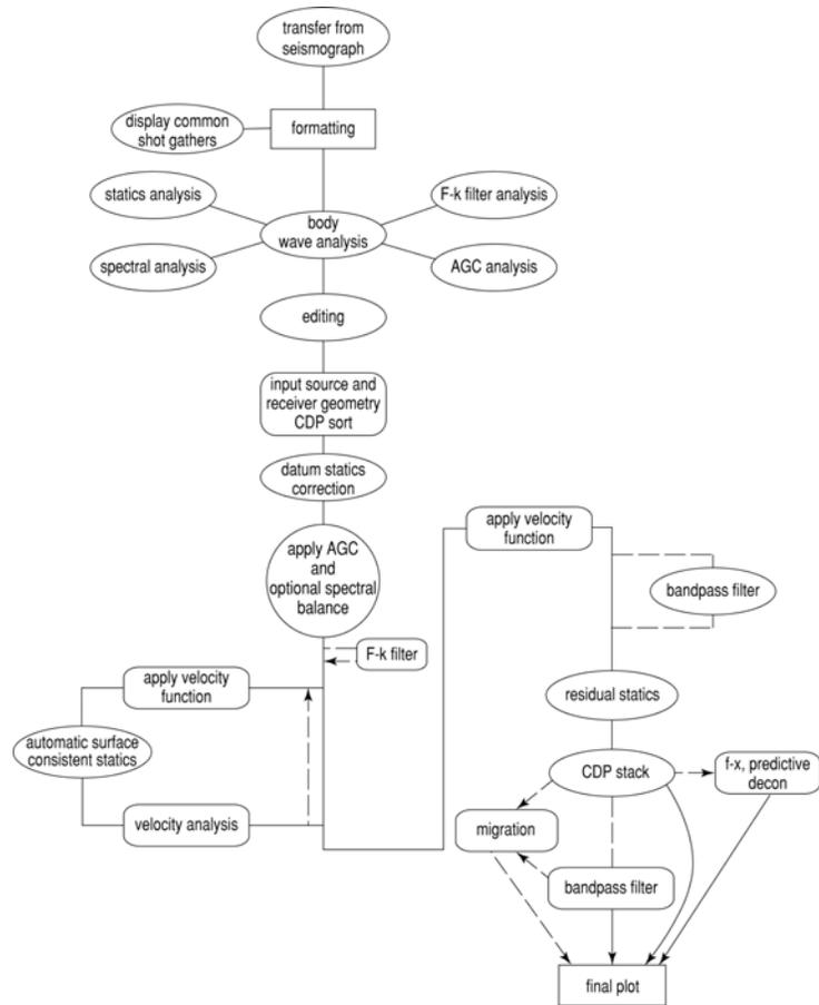
Figure 43. Processing flow for reflection data.
