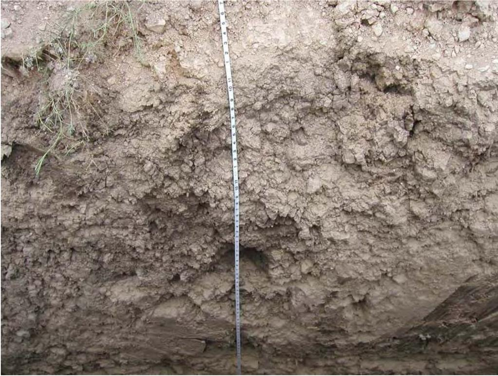
**Top photo:** view of profile RS 5 from surface to about 4.5 ft. Corresponds to northwest portion of above photo showing different layers in levee core. Note the blocky texture and individual clay pieces or pedon surfaces.
