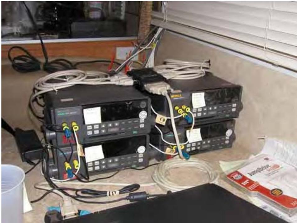
Figure 27. Data recorders used to measure voltages on each SP line of electrodes
