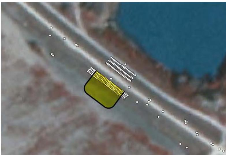
Figure 39. Key stations occupied during 2003 seismic investigation at site 2 with location of pond superimposed.
