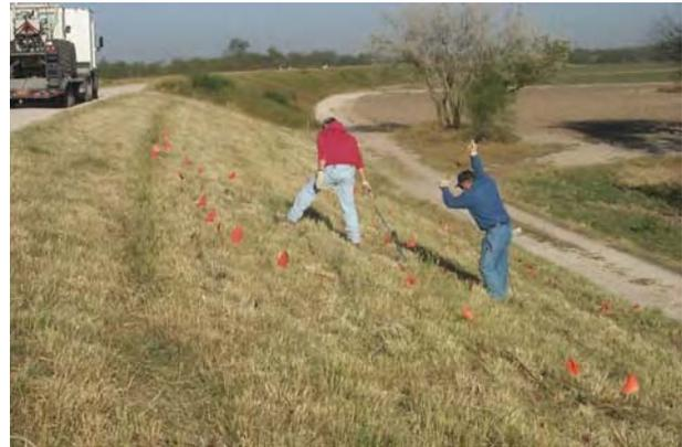
Figure 23. Compressional-wave survey, site 2.
