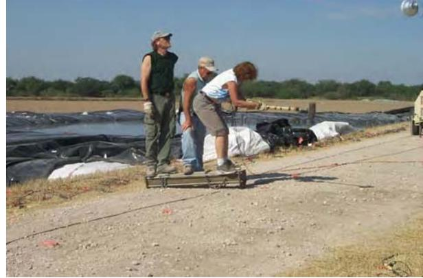
Figure 34. Shear-wave survey during full pool.
