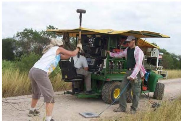
Figure 7. Compressional-wave hammer survey.
