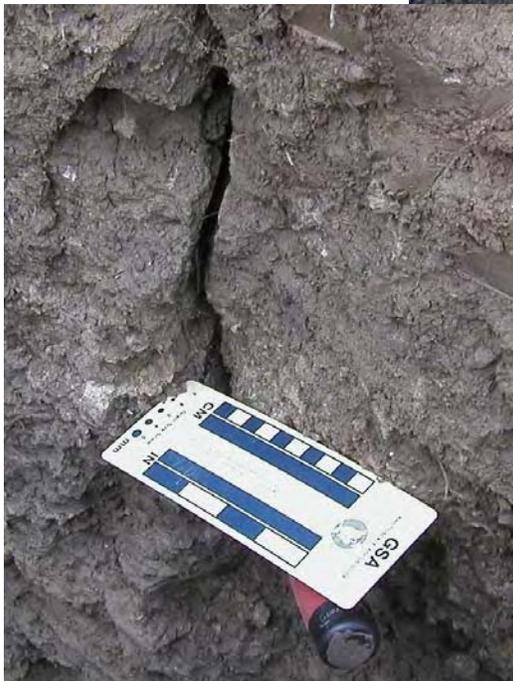
Close up of crack, note blocky texture of soil, and fine sand partings between blocks
