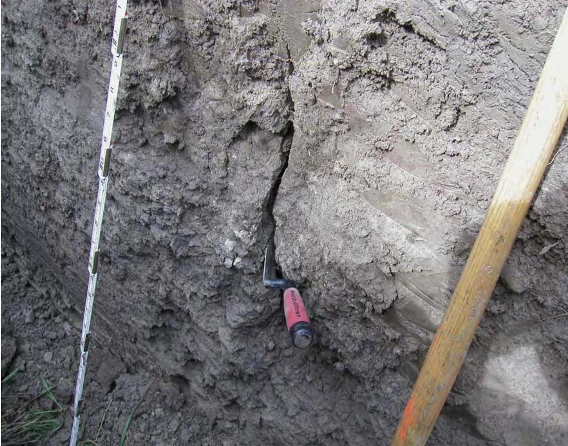
Figure 5. View looking west at profile LS 25 showing crack extending from 2.2 to 3.7 ft,note trowel in vertical crack ranging from ¼ to ½ in. wide.
