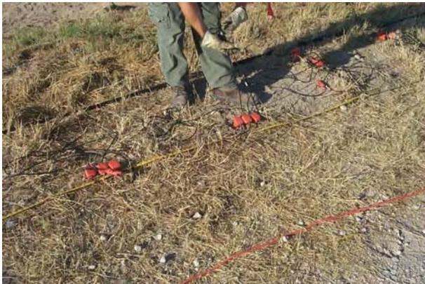
Figure 29. Receiver station spacing was 3 ft.
