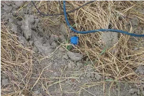
Figure 22. Shear-wave phone.
