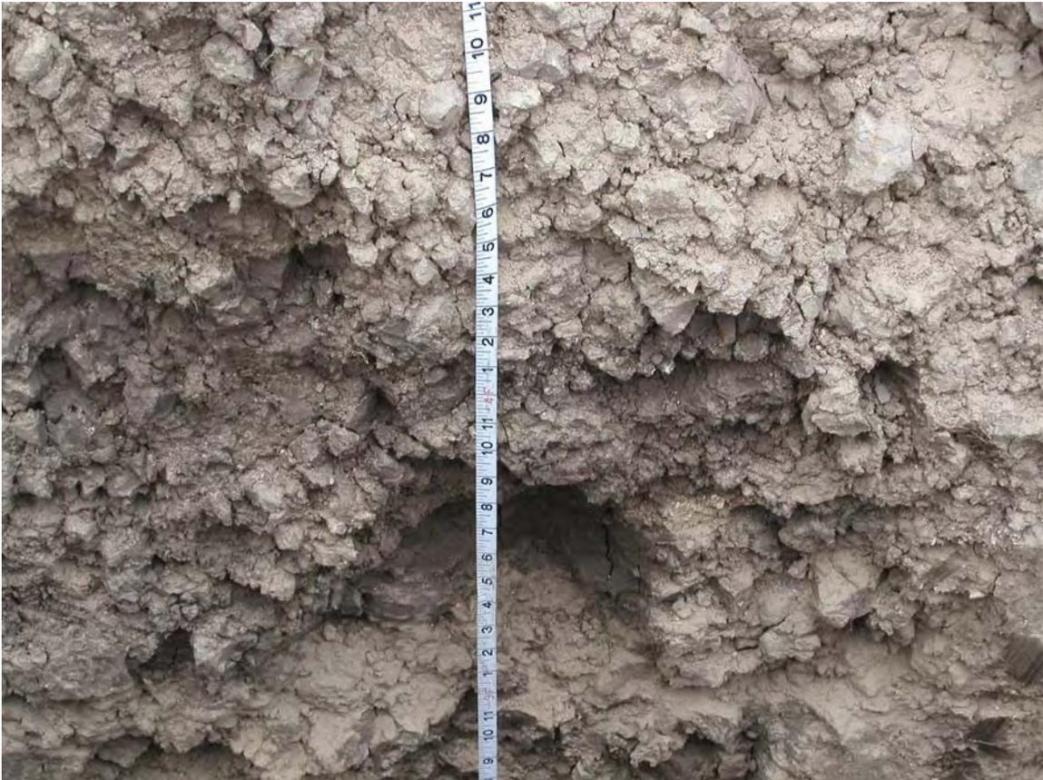
Figure 4. Close-up view looking west at cracked, blocky clay texture at RS 5, depth from about 2 to 3 ft.
