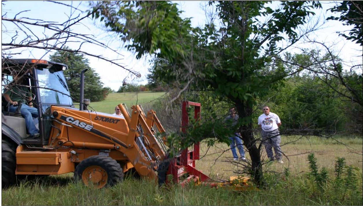
Figure 6. Tree shears are used to control the encroachment of woody vegetation on projects in the Kansas City District (photo courtesy of P. Bailey).
