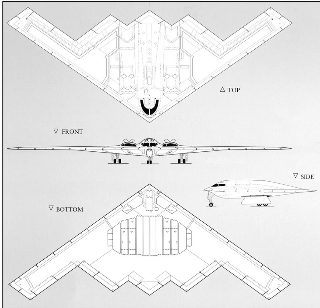
**Figure 1. External View Drawings of the B-2 Aircraft [1]**
