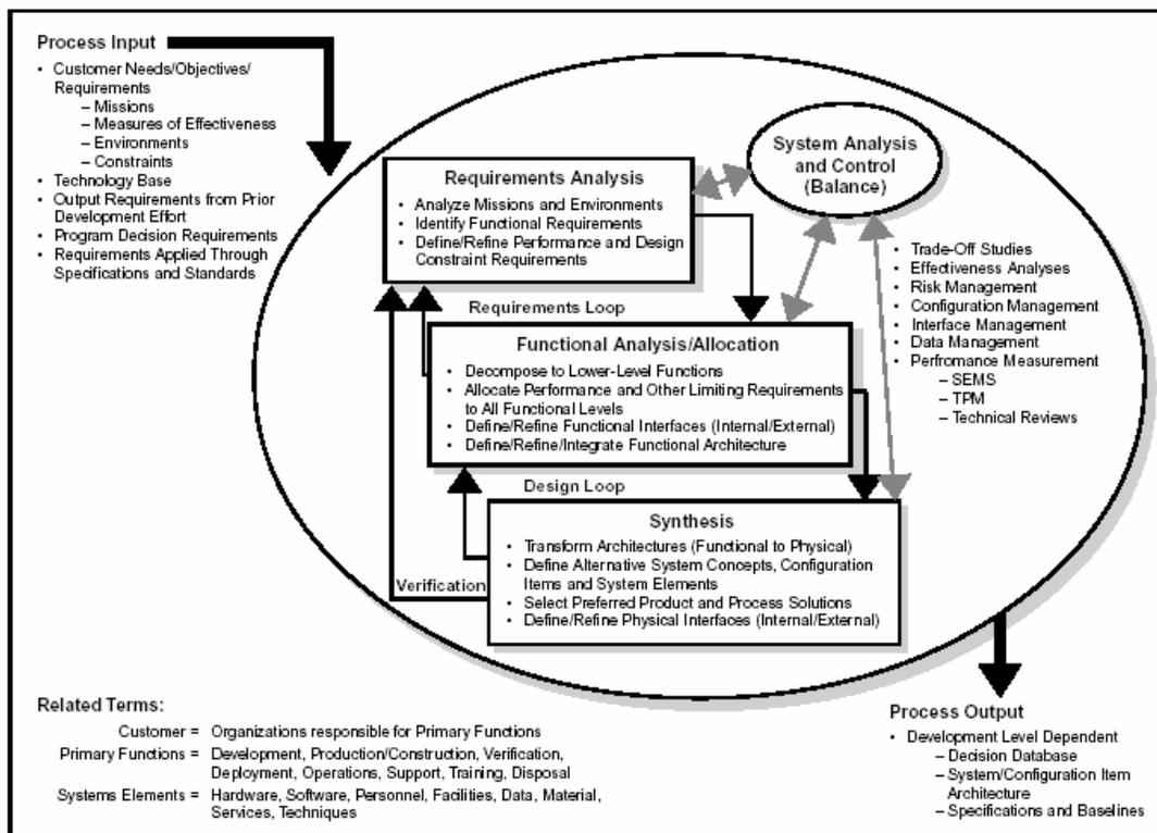
**Figure 1-1. The Systems Engineering Process, Defense Acquisition University**
