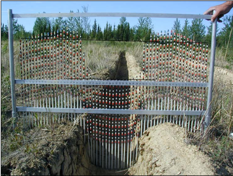
Figure 3. Rut depth measurement and determination using a profilometer.
