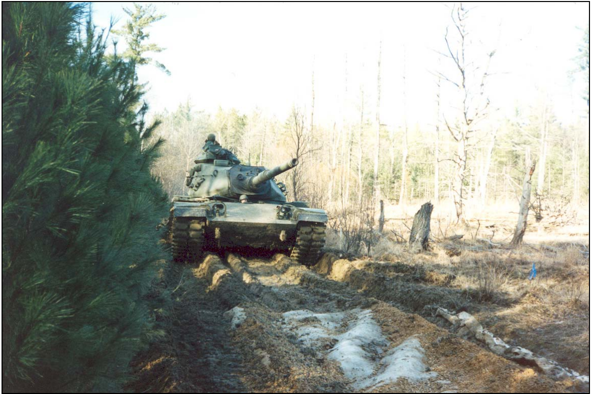
Figure 16. Control section of the wooded trail at Fort McCoy trafficked by an M60A3 in April 1995.
