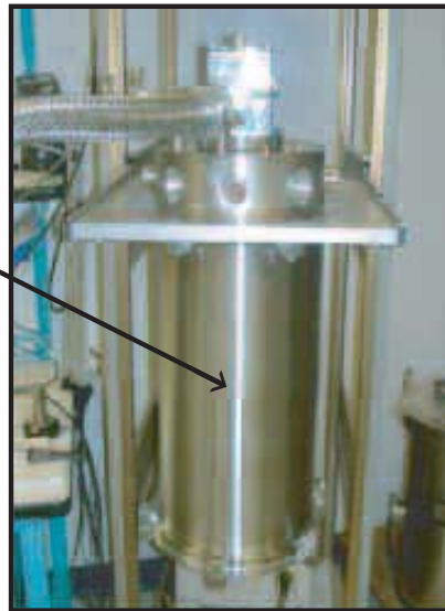
Figure 7. A typical cryocooler enclosure designed for communication applications (Ref: HYPRES).
