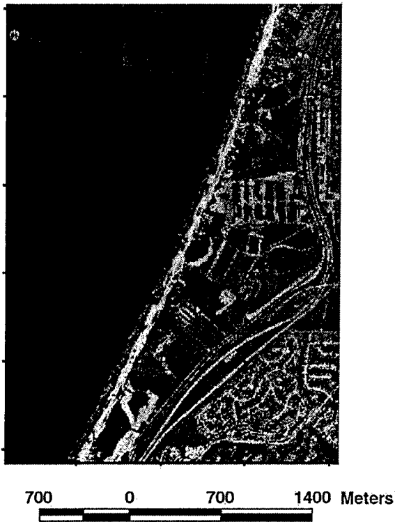
Fig. 4. Elevation differences measured with LIDAR between 1997 and 1998 for 4 km of shoreline centered on Fort Ord. Red and yellow indicate dune erosion, green is no change and blue indicates beach accretion. Large alongshore variations in erosion are indicated.
