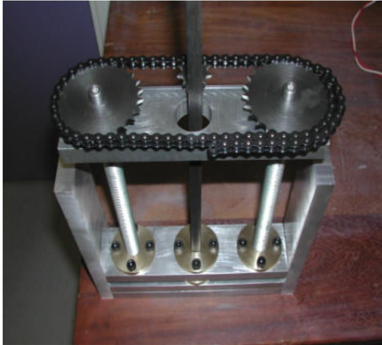
Figure 6. Manufactured Adaptive Stiffness Torsion Bar Concept.
