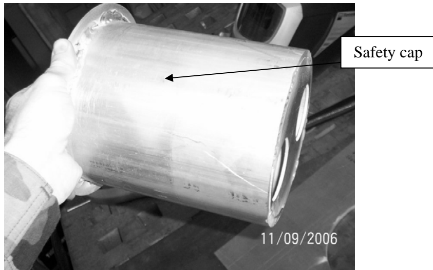
Figure 25. Safety cap without moderators or absorbers.
