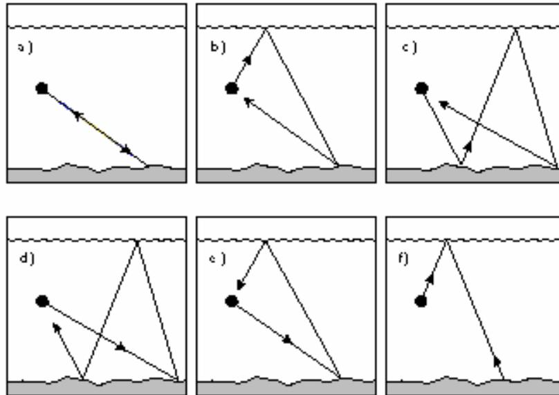
**Figure 3: Diagram showing the direct path measurement technique and the various paths for acoustic energy (path a – direct path source to bottom and back to receiver, path b – path from source to surface, bottom and receiver, etc.).**
