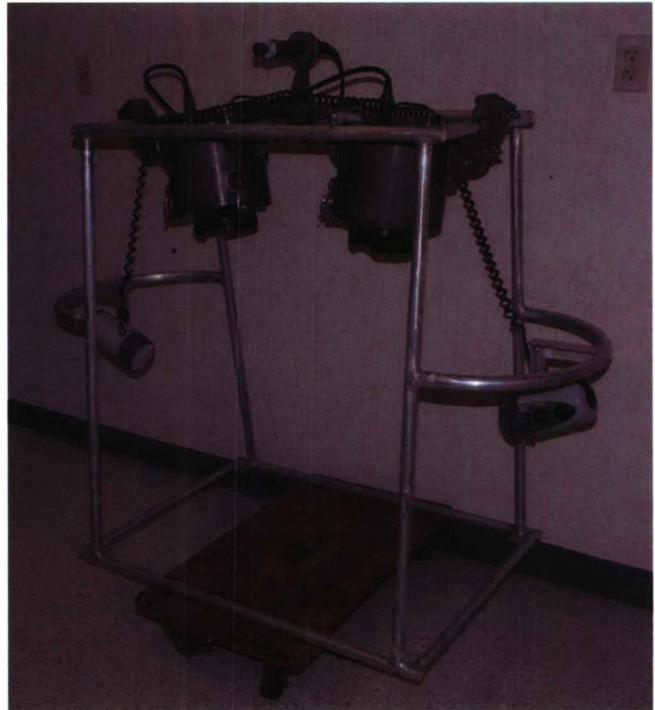
Figure 1. The NRL digital stereo camera system mounted on a tubular aluminum frame and including two Ikelite strobes mounted outboard of the 95×67-cm overlap field of view.
