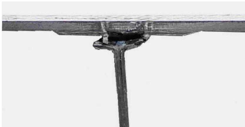
Figure 6.1.1.3: Specimen 1c after dynamic test
