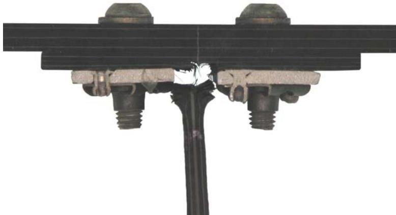
Figure 6.2.1.5: Specimen 2e after dynamic test.
