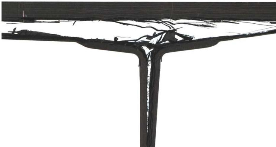
Figure 6.3.1.2: Specimen 3b after dynamic test
