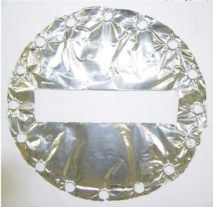
Figure B.1: Typical failure of an aluminum diaphragm.
