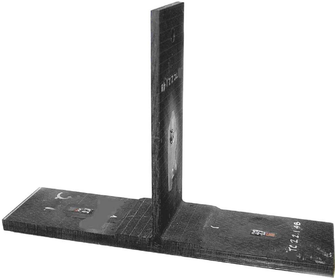
Figure 6.3.2: Example image of joint from Specimen Set 3 (pretest)
