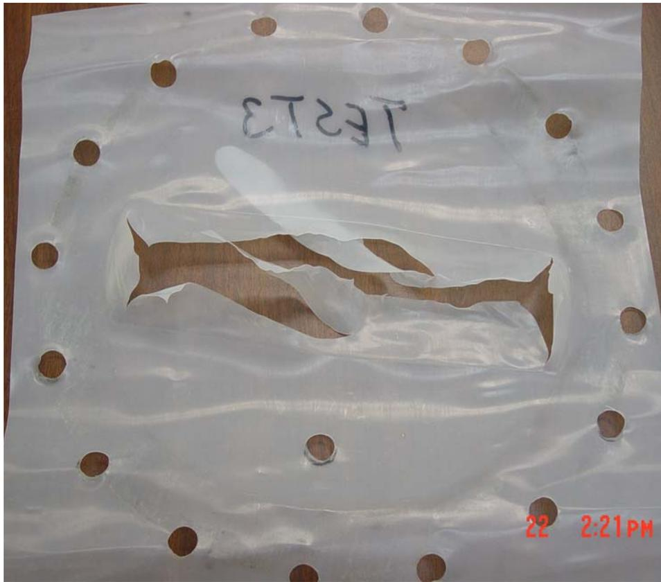
Figure B.2: Typical failure of a UHMWPE diaphragm (0.015 thick).
