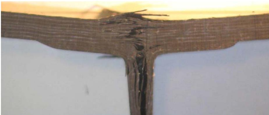
Figure 6.3.2.3: Specimen 3h after static test.
