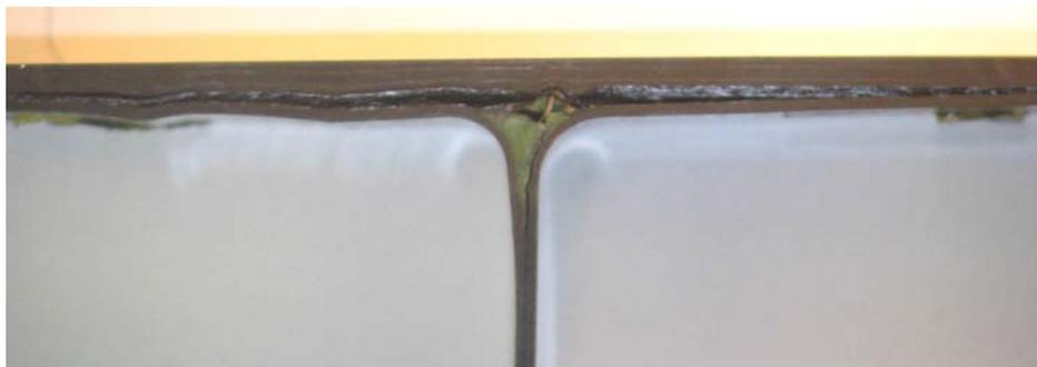
Figure 6.7.2.2: Specimen 7g after static test.
