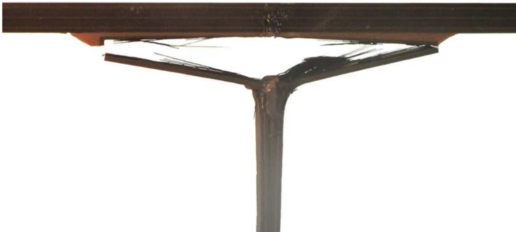
Figure 6.9.1.3: Specimen 9c after dynamic test
