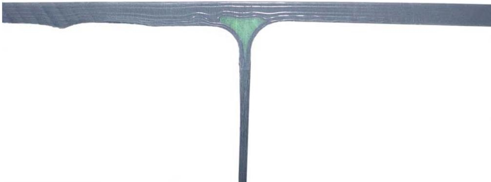
Figure 6.7.3: Example cross section of joint from Specimen Set 7 (pretest)
