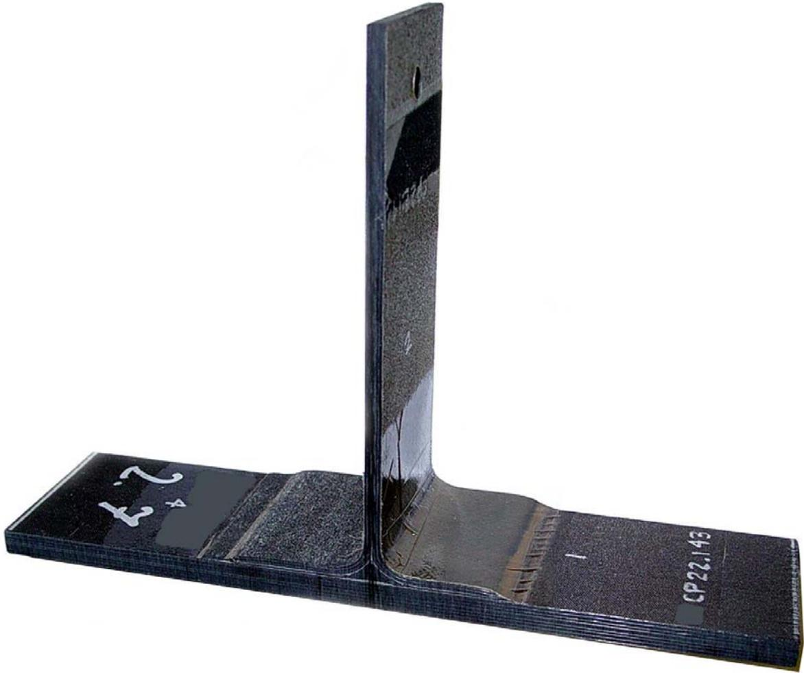
Figure 6.5.2: Example image of joint from Specimen Set 5 (pretest)
