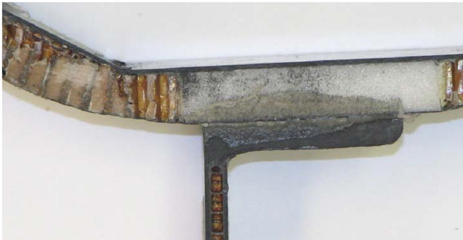
Figure 6.10.2.4: Specimen 10g after static test.
