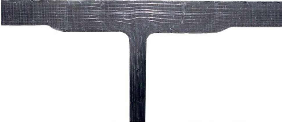
Figure 6.3.3: Example cross section of joint from Specimen Set 3 (pretest)
