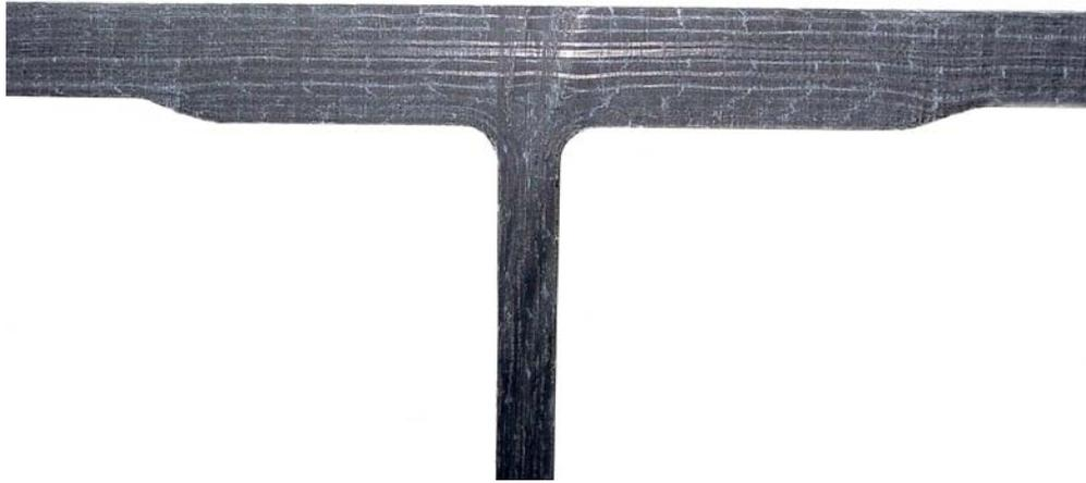
Figure 6.6.3: Example cross section of joint from Specimen Set 6 (pretest)
