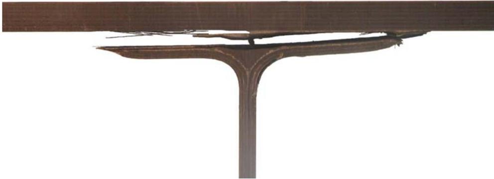
Figure 6.5.1.2: Specimen 5b after dynamic test
