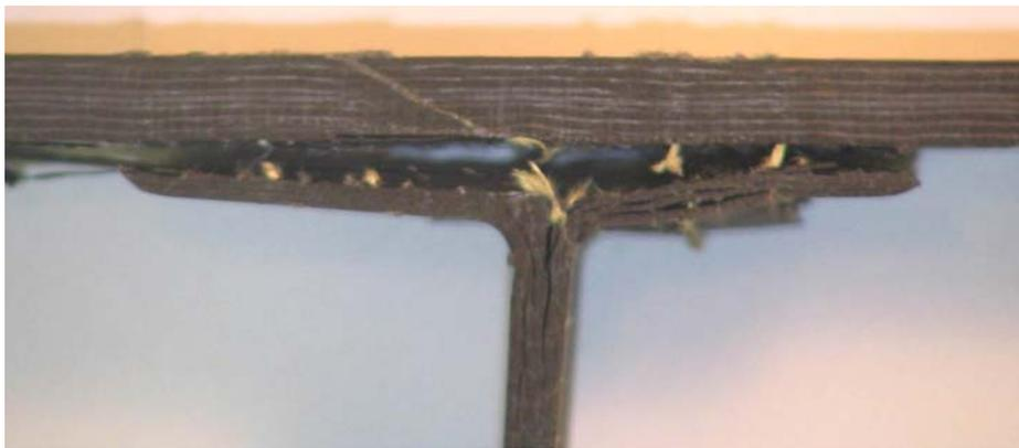
Figure 6.4.2.1: Specimen 4f after static test.
