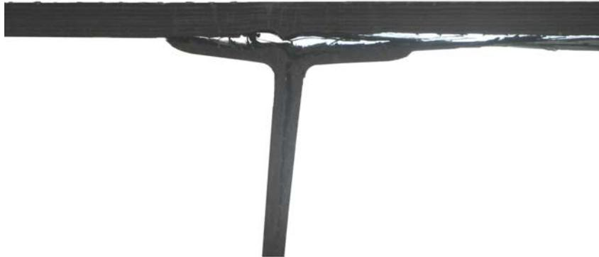
Figure 6.3.1.3: Specimen 3c after dynamic test
