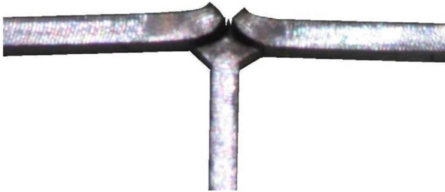
Figure 6.8.1.2: Specimen 8b after dynamic test
