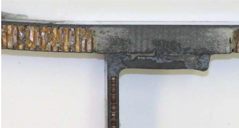
Figure 6.10.2.5: Specimen 10h after static test.
