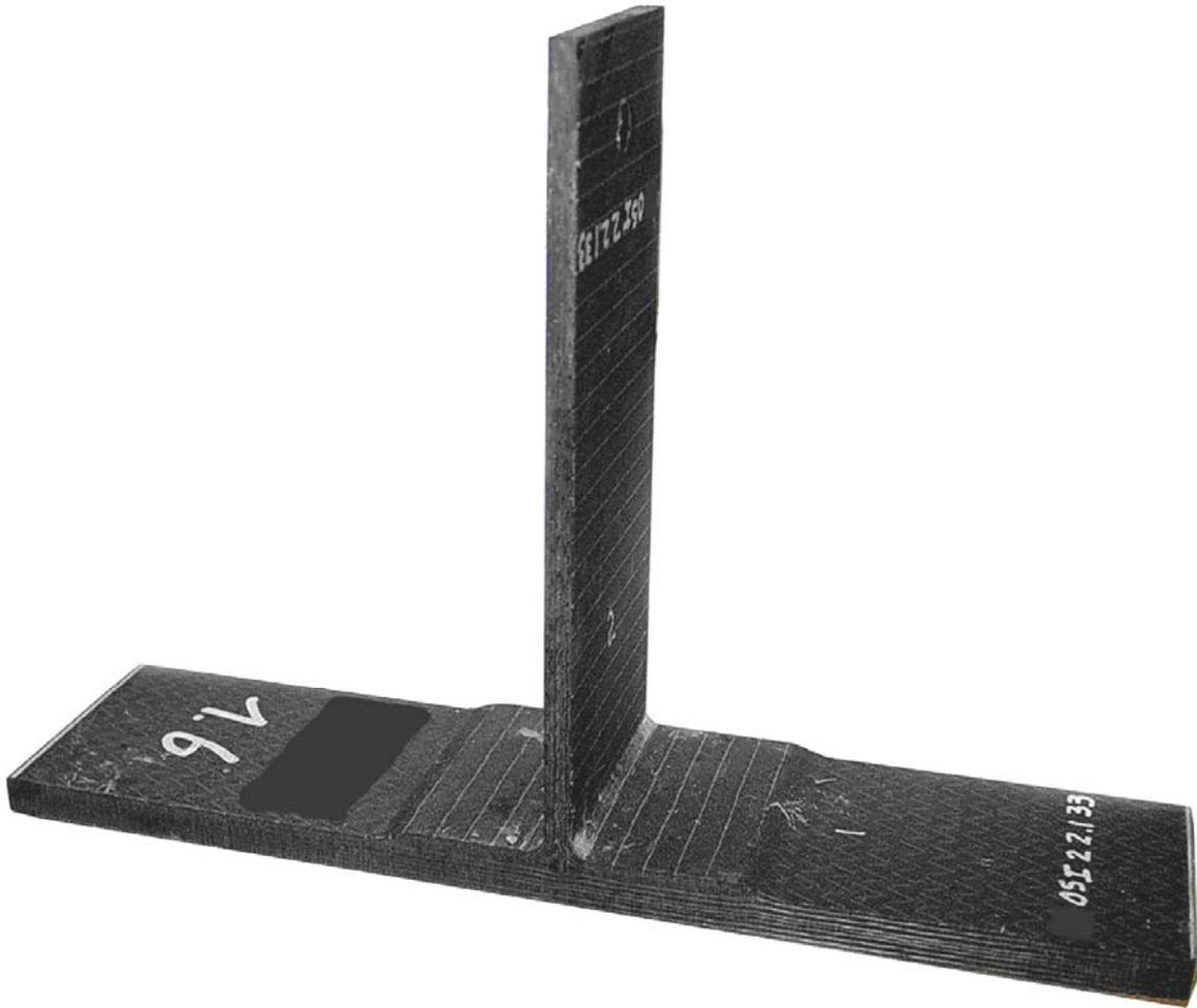
Figure 2.2: Example single spar T-joint
