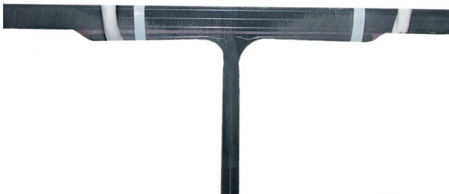
Figure 6.9.3: Example cross section of joint from Specimen Set 9 (pretest)
