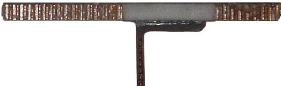
Figure 6.10.3: Example cross section of joint from Specimen Set 10 (pretest)
