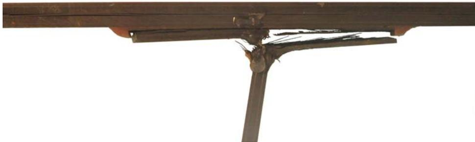
Figure 6.9.1.1: Specimen 9a after dynamic test
