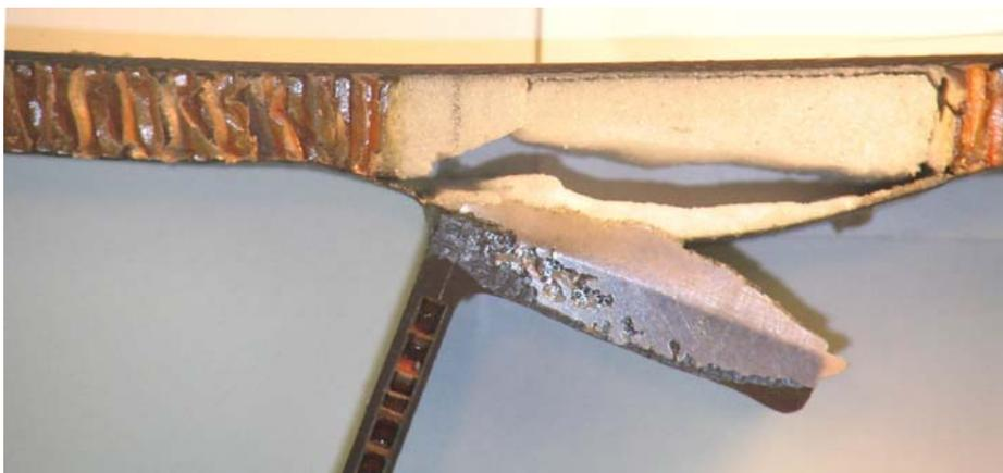
Figure 6.10.2.2: Specimen 10e after static test.
