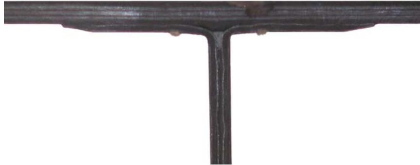
Figure 6.1.1.4: Specimen 1d after dynamic test.
