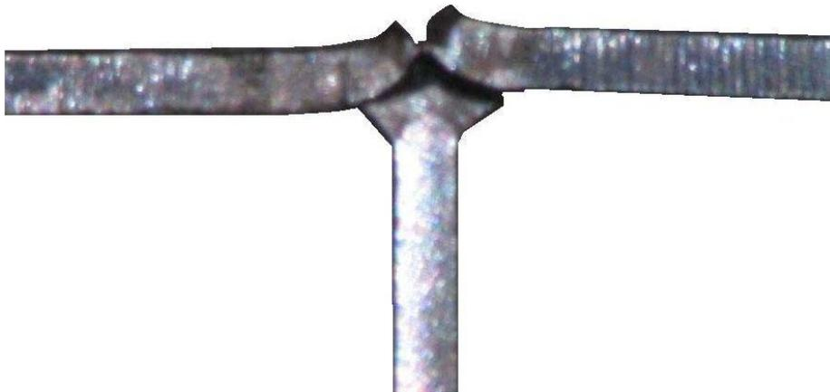
Figure 6.8.1.3: Specimen 8c after dynamic test
