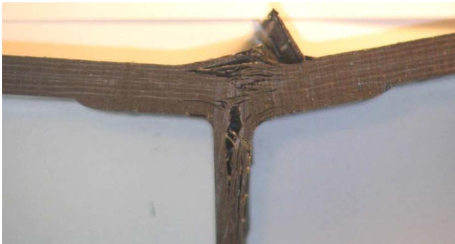
Figure 6.3.2.5: Specimen 3j after static test.
