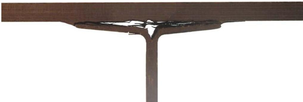
Figure 6.6.1.3: Specimen 6c after dynamic test
