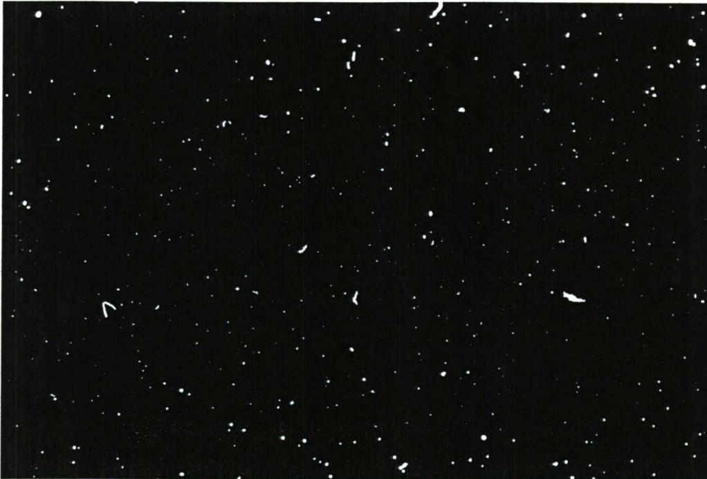
Figure 18. Digital photo image of normal dust on a silicon wafer. Photo is at closest focusing distance for 100-mm macro lens.
