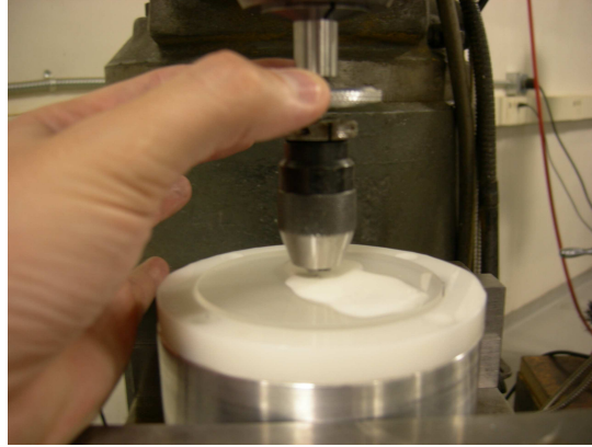
Figure 4.8: Lapping tool mounted in zero-force chuck
