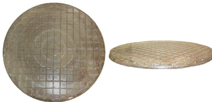
Figure 4.3: Typical channeled pitch tool (12 inch diameter)
