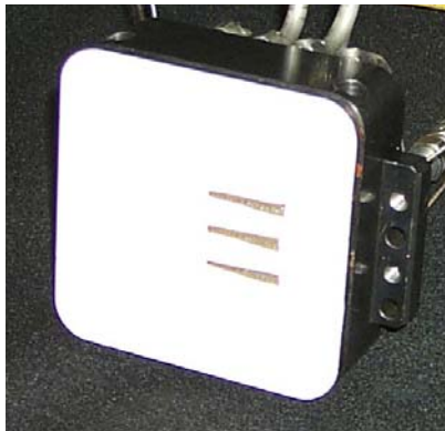
Figure 2: Aerojet cascade injector block
