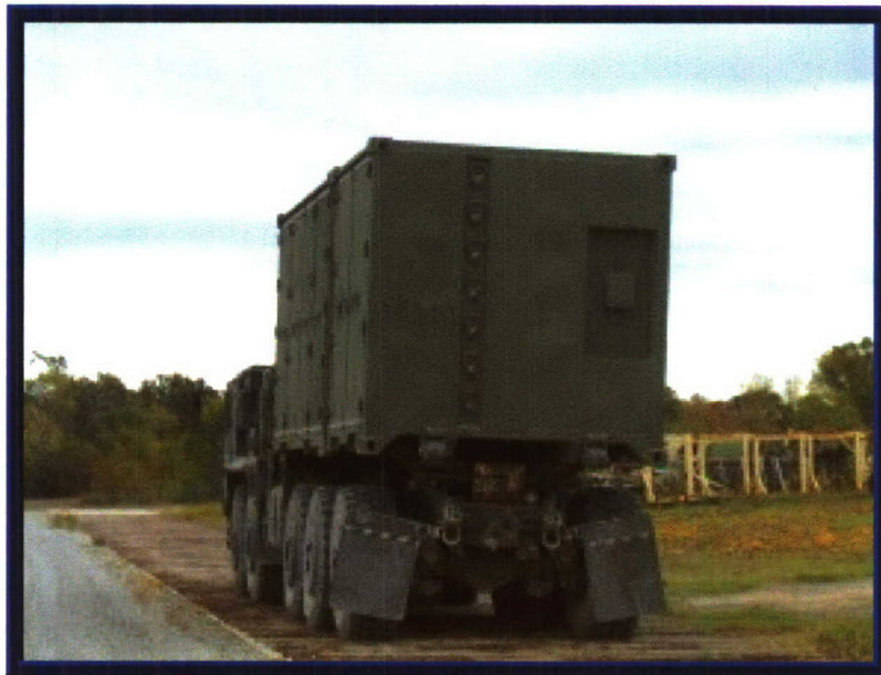
Photo 10. Washboard Course Testing of the Coupled BOH Containers on the PLS Vehicle.
