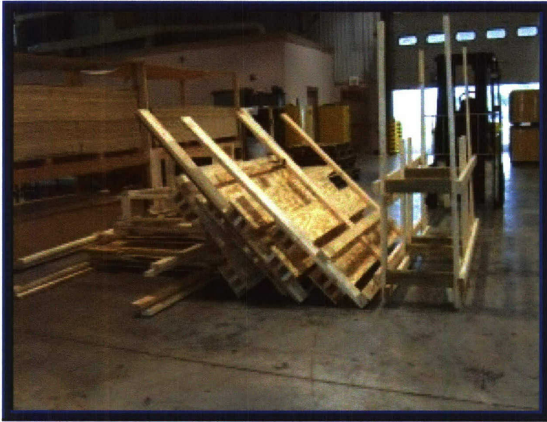
Photo 12. Dunnage Required to Secure Payload.
