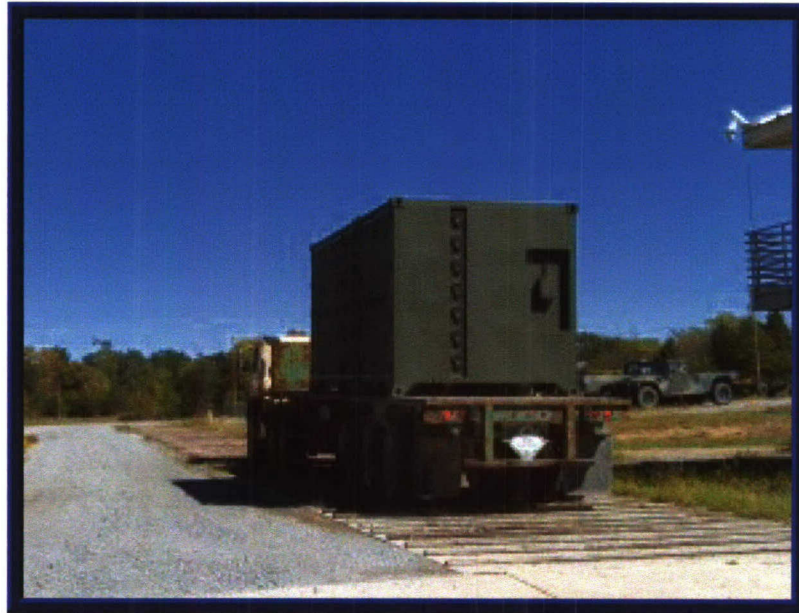
Photo 6. Washboard Course Testing of the Coupled BOH Containers.
