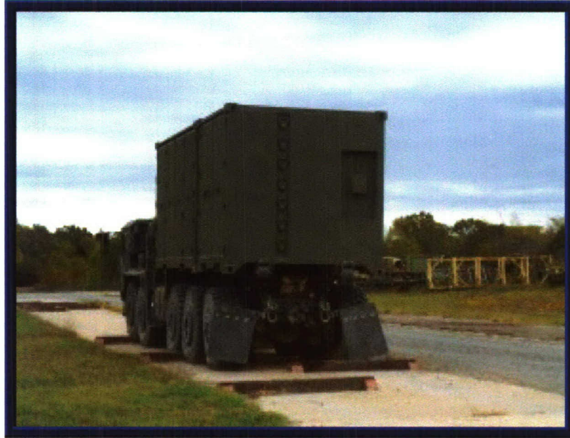
Photo 8. Hazard Course Testing of the Coupled BOH Containers on the PLS Vehicle.
