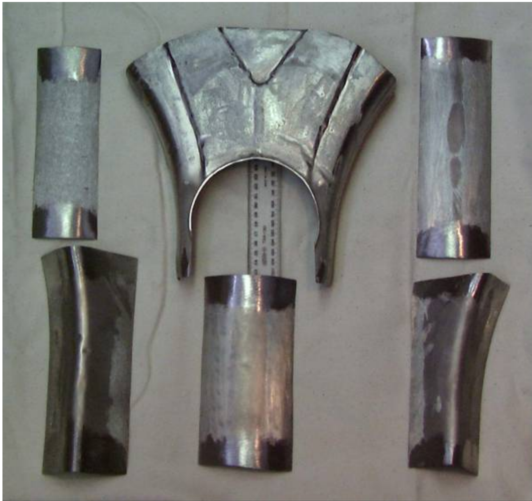
Figure 10 Electroformed reinforcements, clockwise from the top left regions D, A, E (outer) and B, E (inner) and C
