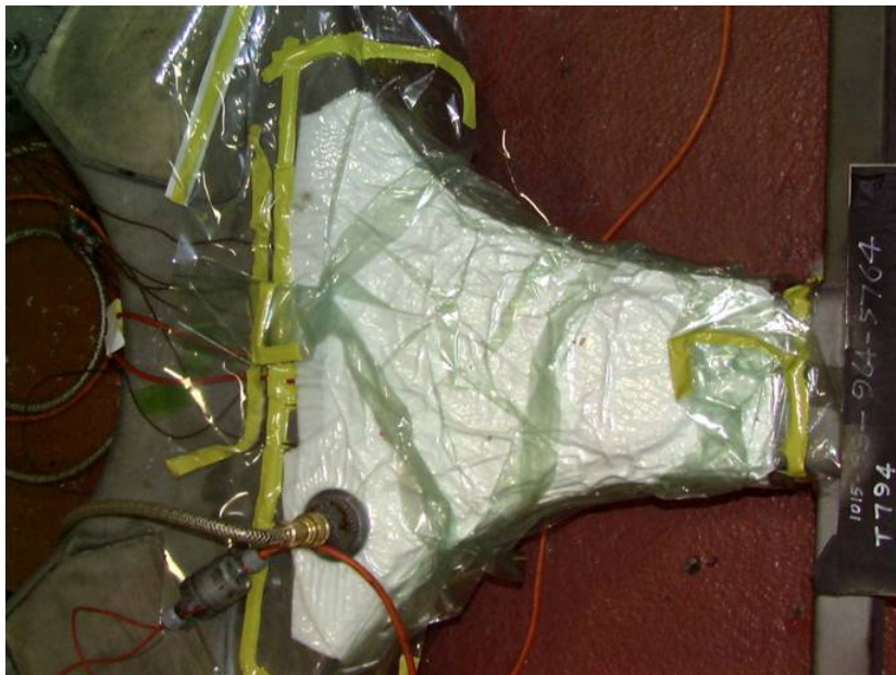
Figure 14 Application of the reinforcement region A in the boss region, showing vacuum bagging assembly
