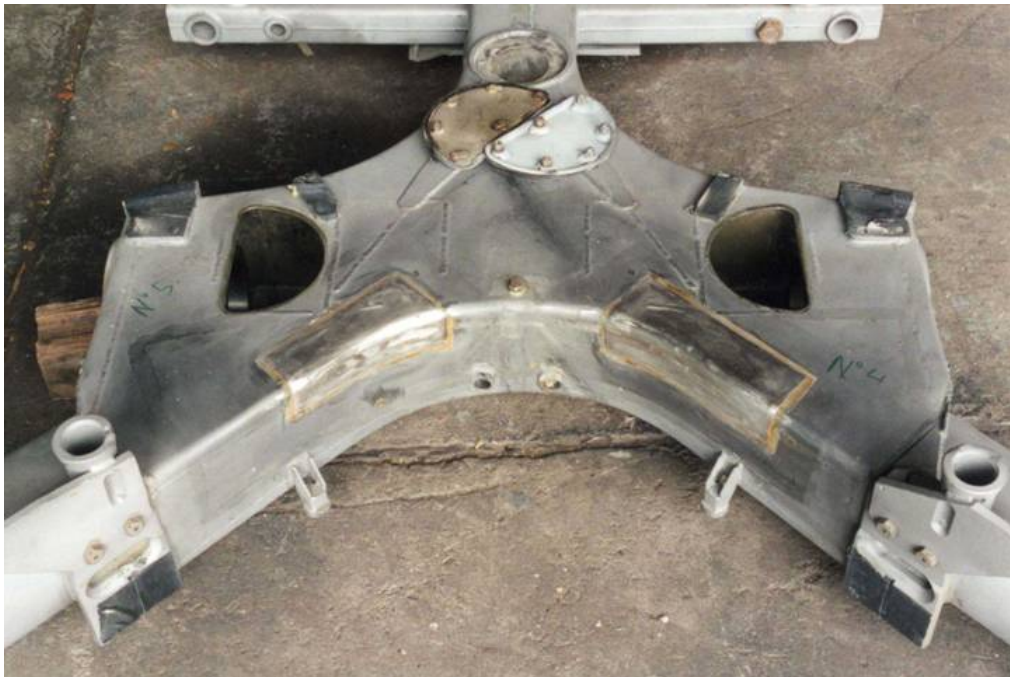
Figure 17 Reinforcements bonded to region C (left and region B right
