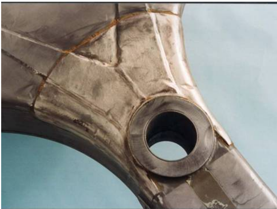
Figure 16 Reinforcement bonded to boss region A
