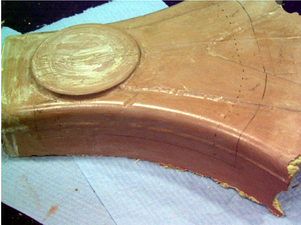
Figure 9 Glass/epoxy mould for electroforming the nickel reinforcement for the boss region of the trail
