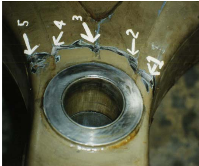
Figure 2 Gun trail showing severe chain scored region ~ 20 mm from boss rim; the region is shown circled in Figure 1- the arms extend from the top of this photograph
