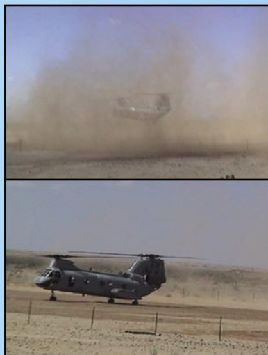
Catastrophic dust abatement using NRL-DAS6100 formulation.
