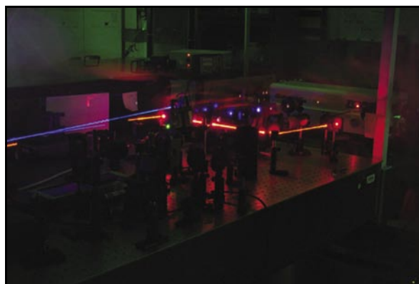
Femtosecond laser system for ultrafast dynamics; nonlinear mixing techniques are used to generate femtosecond pulses over a wide range of wavelengths. These techniques include photochemistry and vibrational energy dynamics of ions in solution and in reverse micelles.
