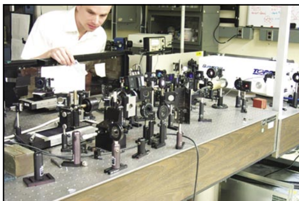
Femtosecond laser system for ultrafast dynamics; nonlinear mixing techniques are used to generate femtosecond pulses over a wide range of wavelengths. These techniques include photochemistry and vibrational energy dynamics of ions in solution and in reverse micelles.
