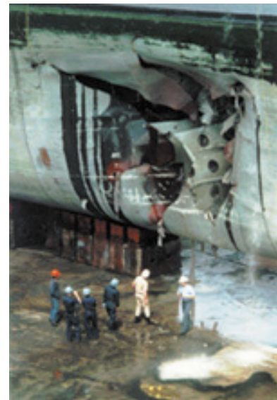
Figure 2 Damage done to TRIPOLI by a single mine
