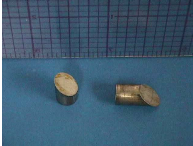
FIGURE 2. 30 Caliber “Wedge Projectile” used in Task 3 Ballistic Experiments
