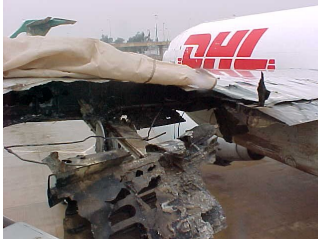
Photo of wing damage after MANPAD attack (Airbus Industries Photo) 22 Figure 2
