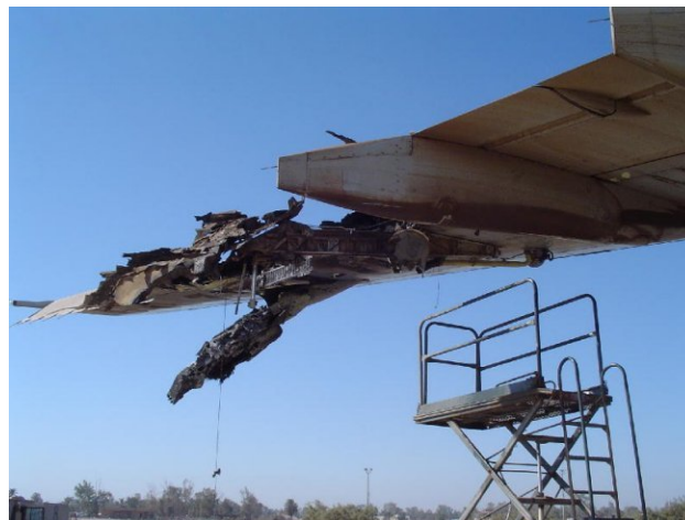
Photo of wing damage after MANPAD attack (Airbus Industries Photo) 23 Figure 3
