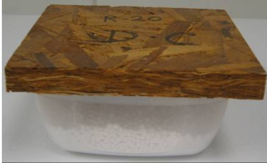
Figure 2. Test setup for water vapor transmission and permeance measurement.
