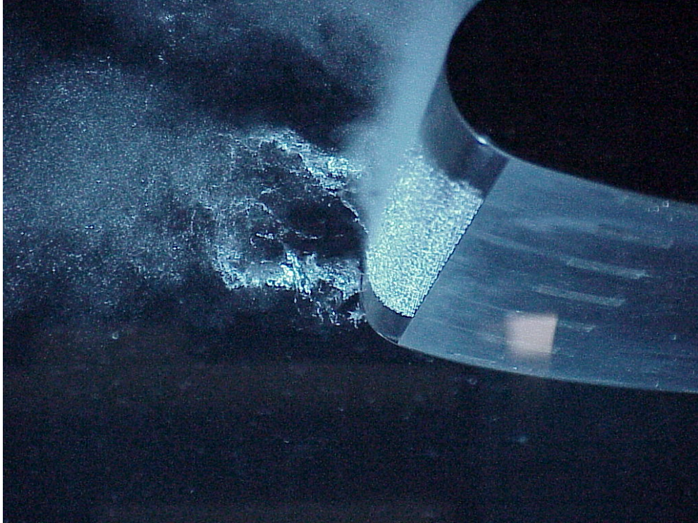
Figure 71. Surface Cavitation on Coanda Surface, lower slot blowing.
