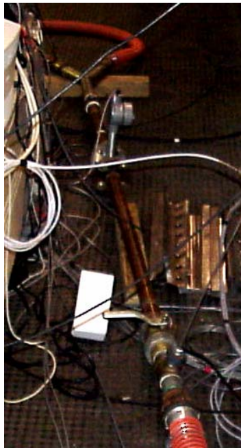
Figure 15. Flow Measurement layout showing Hoffer turbine flowmeter
