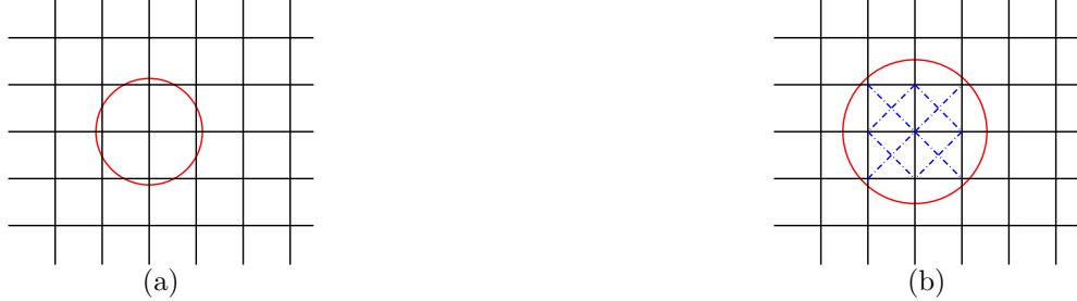
Figure 5: The effect of ratio \kappa on validity of a square lattice as an \alpha -lattice: (a) \kappa = 1 + \varepsilon < \sqrt{2} (valid) and (b) \kappa = \sqrt{2} + \varepsilon (invalid).
