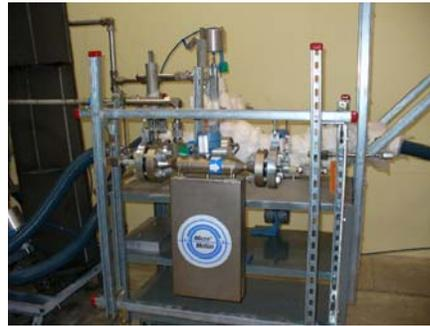
Figure 14: Regulator and mass flow meter
