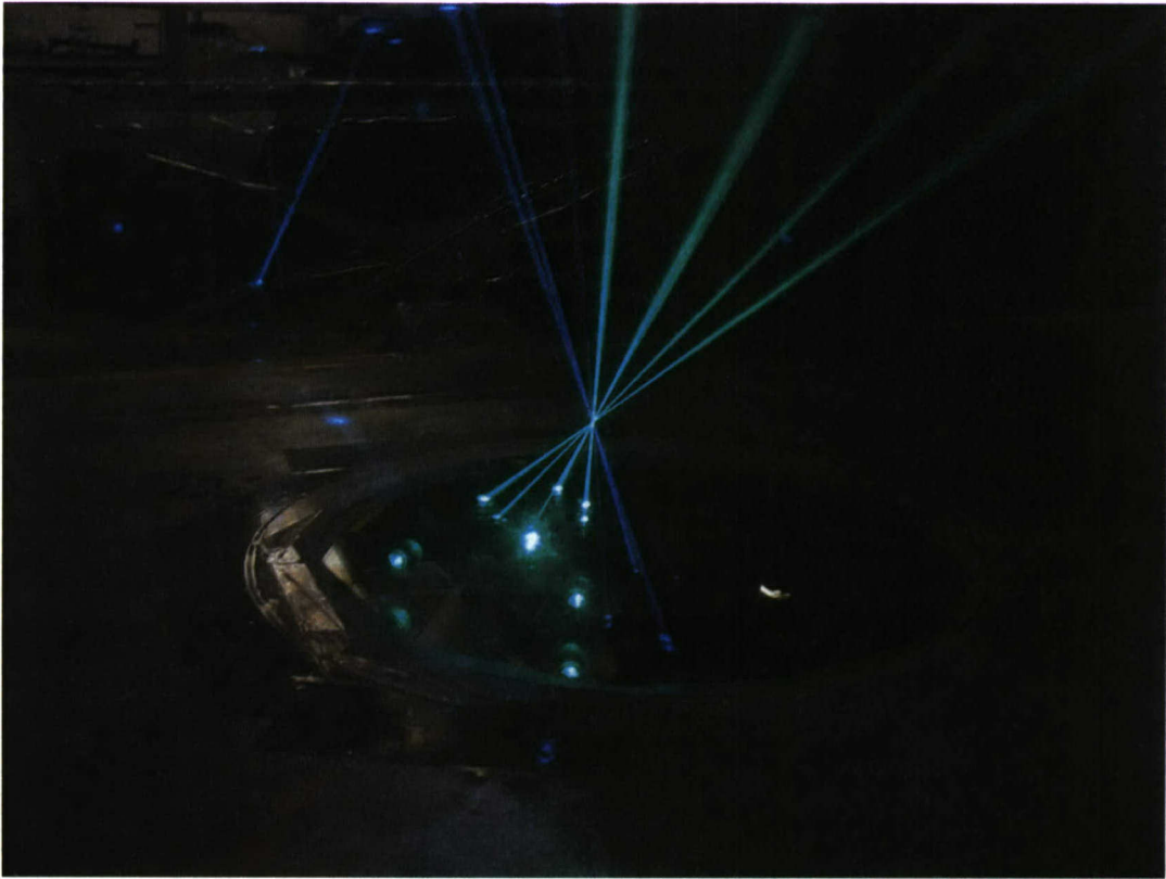
Figure 2.8. Photograph of laser beam configuration for the CompLDV3.
