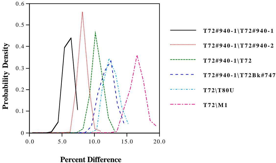
**Figure 3.** The probability density displayed as a function of the APD correlation for MBT Ka-band scaled-signature ISAR.
