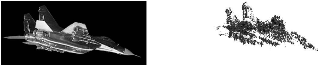
Figure 10. Mig29 48 th scale model (left) and Az/EI image (right) at negative 15° elevation, 235° aspect, 35 GHz (Ka-band) HH polarization, 2" full-scale resolution.
