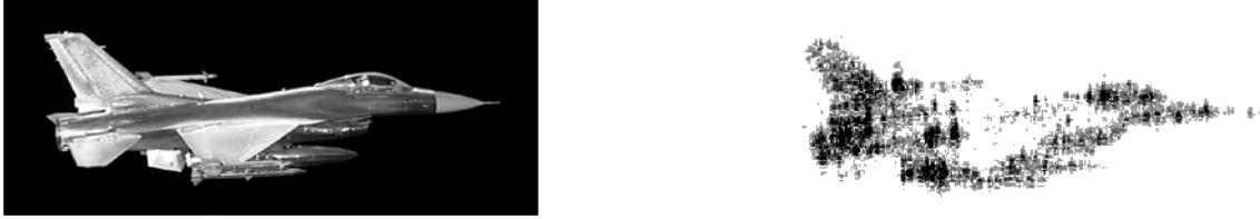
Figure 8. F-16 48 th scale model (left) and Az/EI image (right) at 15° elevation and 260° aspect, 35 GHz (Ka-band) HH polarization, 2" full scale resolution.
