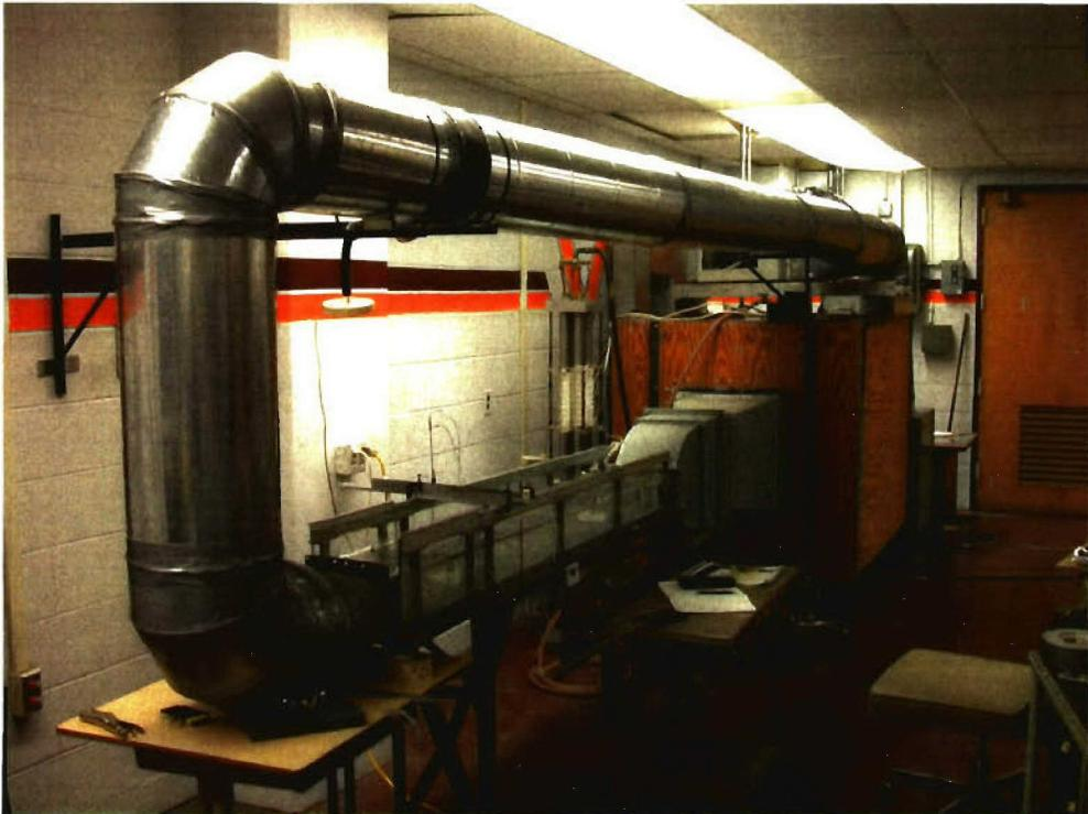
Figure 2.2: Small boundary layer wind tunnel setup (view from front)
