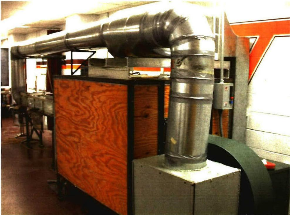
Figure 2.3: Small boundary layer wind tunnel setup (view from back)
