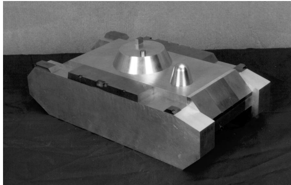
Figure 8. The complex target simulator (CTS) shown from a rear quarter view.
