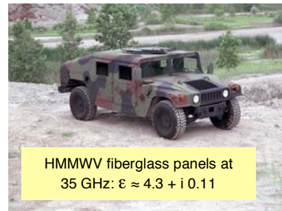
Figure 1. Complex dielectric constant of a D-38 loaded artificial dielectric at 0.52 THz (left) and the 35 GHz properties of fiberglass (right).
