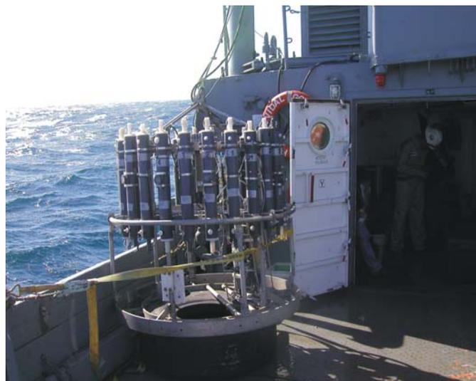
Figure 10: A water sampling rosette equipped with a depth finder, CTD probes and 24 1-L Niskin bottles were used to sample the water column for methane transported from the sediments.
