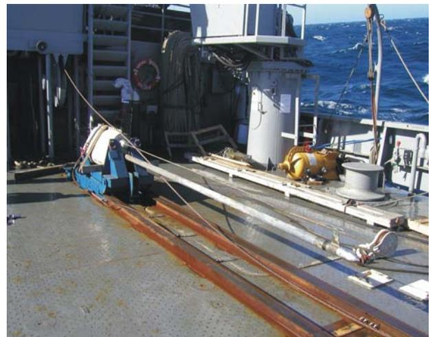
Figure 8: NRL's marine heat-flow probe system, designed and built by the Geological Survey of Canada, is designed to measure temperature gradients and in-situ thermal conductivity of sediments.
