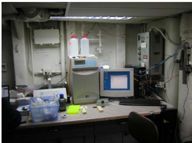
Figure 7a: Ion chromatograph used to measure sulfate and chloride concentrations in porewater.
