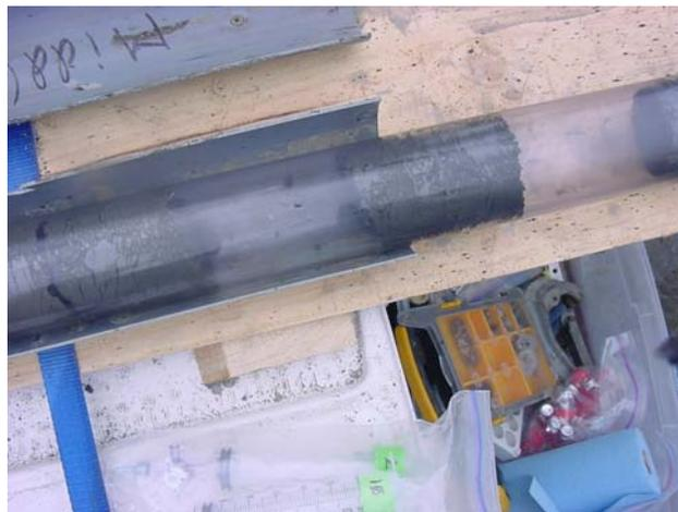
Figure 6: Cores sleeves were taken from the piston core system and prepared on the deck for the porewater press, onboard analysis and sample storage.
