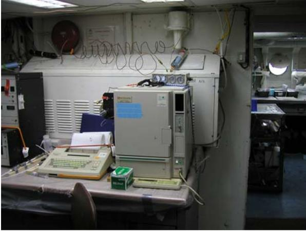
Figure 7c: A gas chromatograph used to measure methane concentrations in porewater.
