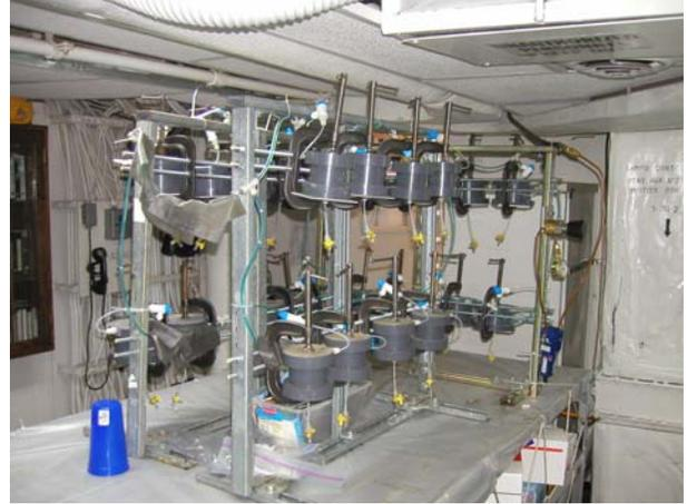
Figure 7d: A 24 port sediment press system to obtain porewater samples.
