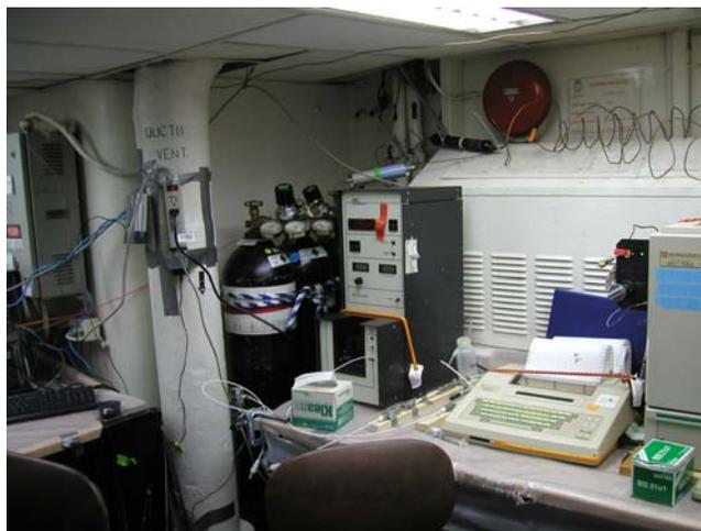
Figure 7b: Coulometer used to measure porewater DIC concentrations
