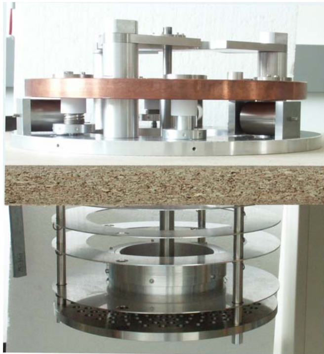
Figure 2.3-4 Copper Ring-Flange Assembly (With Shaft and Superconductor Support Structure)
