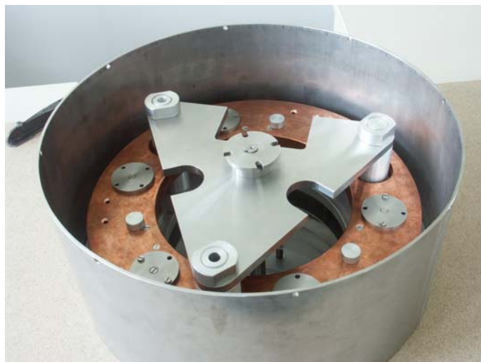
Figure 2.4-1 Motor Axis, Bearing and Coupling Assembly
