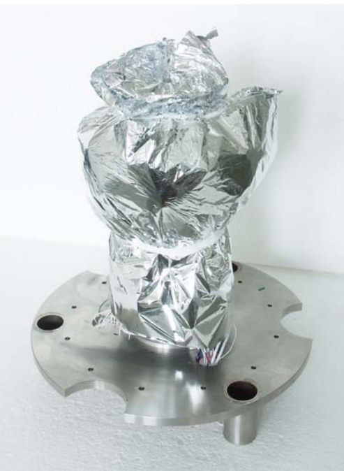
Figure 2.2-2 Complete Assembly of Accelerometers, Heaters, PT-100s and Magnetic Field Sensor on Structure (Left) and Wrapped in MLI Insulation (Right)
