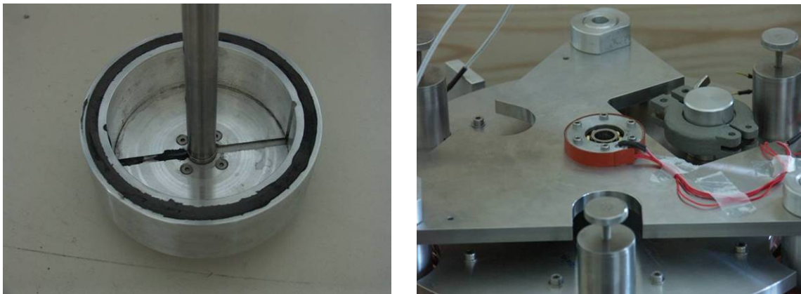
Figure 2.5-1 Superconductor Support (Left) and Upper Bearing (Right)
