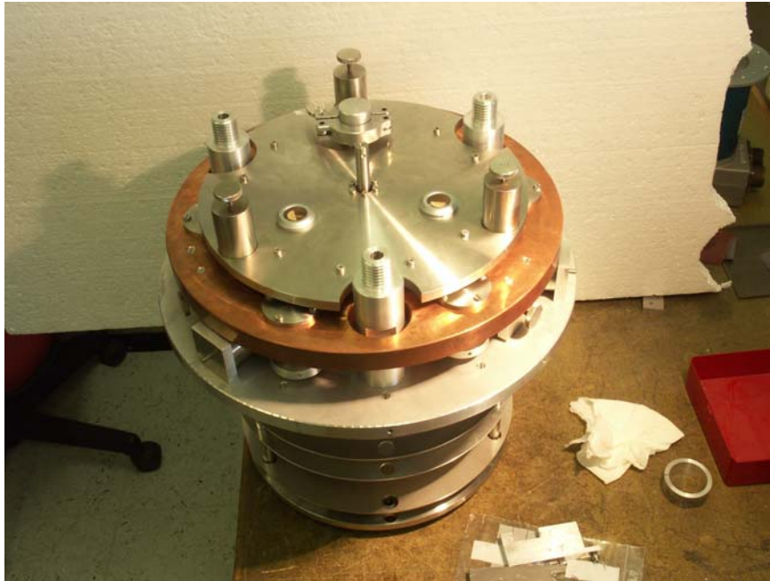
Figure 2.3-5 Complete Damping System Assembly
