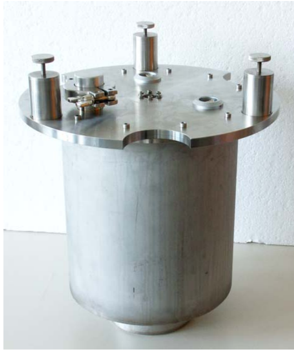
Figure 2.2-3 Completely Assembled Vacuum Chamber
