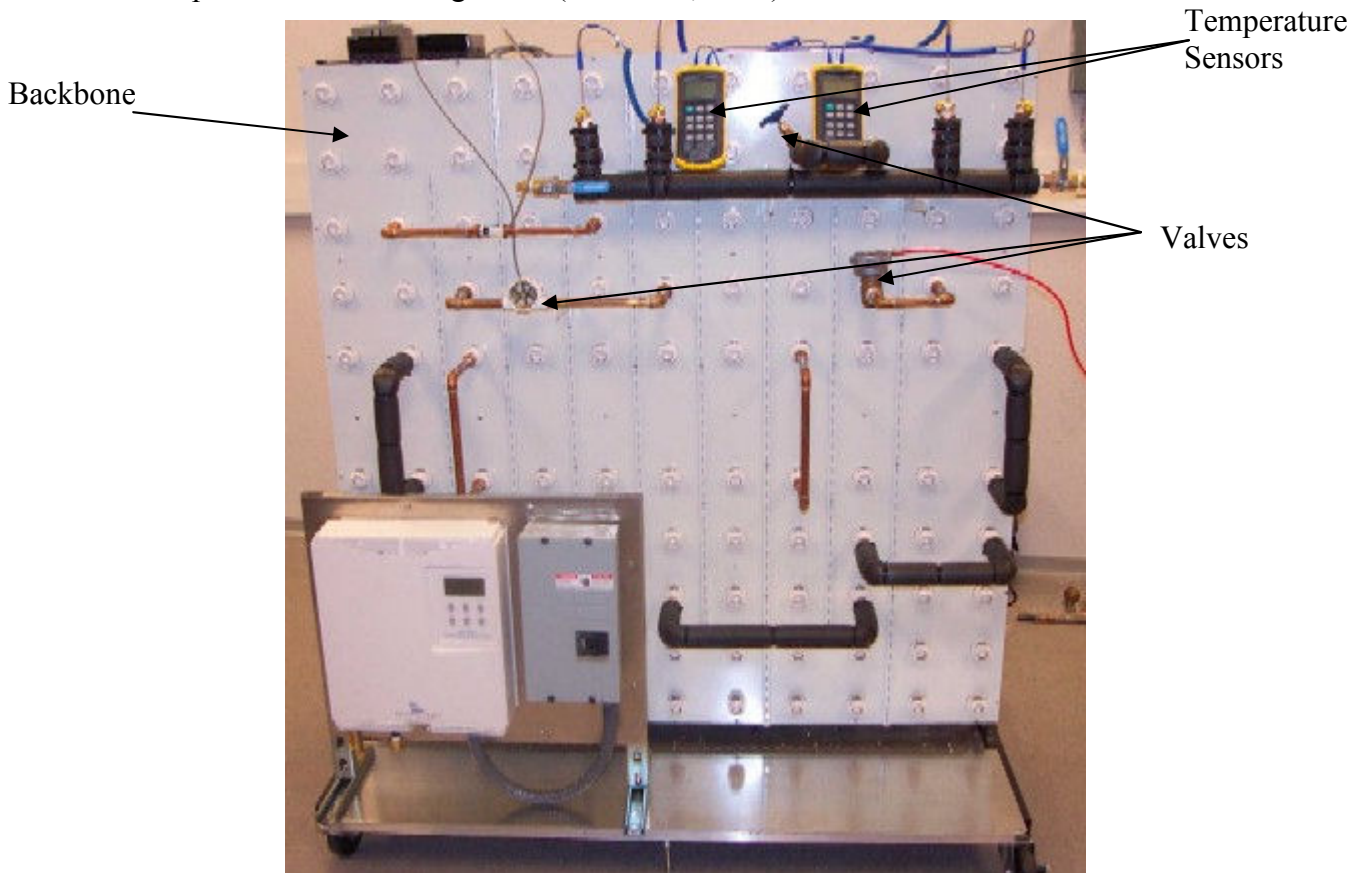
Figure 17: Dr. Mountain's Process Control Breadboard (Mountain, 2004)
