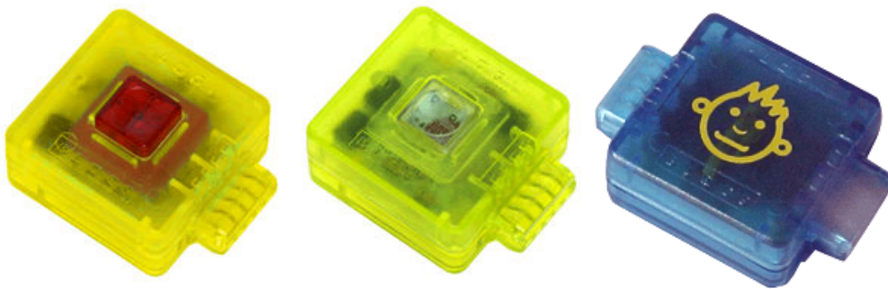
Figure 27: Button, Switch, and Connector Logiblocs ( www.Logibloc.com , 2006)
