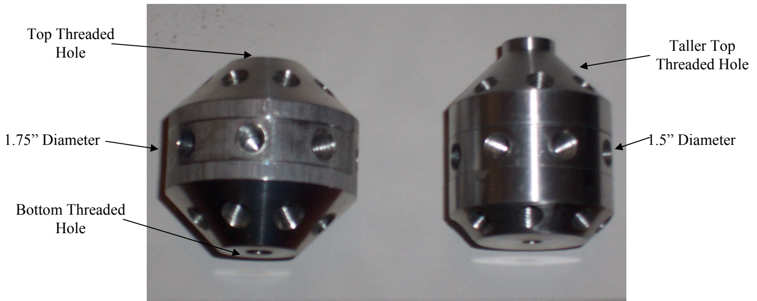
Figure 40: 3rd (left) and 2nd (right) Prototypes
